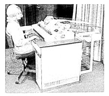
(4) a display above the keyboard which guides the operator through procedural steps and locks the machine if and signal is ignored, forcing corrective action.
