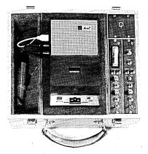
FM record/reproduce electronics and has push button calibration. Designated the Model 7001 Instrumentation Recorder, it has provisions for visual, audible or external monitoring of record/reproduce mode data signals, and the operator may insert voice comments as desired. Applications include recording and analysis of data associated with shock, vibration, noise, pollution, automation, information display, telecommunications, plant maintenance, process variables and medical research.
