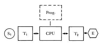
Figure 4. Arrangement where an item of electronic equipment serves as a "student" in a student-to-student computer-mediated interaction.
