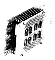
Printed circuit board construction is used throughout and sub-miniature diodes are employed. The new series are particularly adaptable for high density packaging applications in mini- and midi-computers due to each plane being double-matted. (For more information, circle #45 on the Reader Service Card.)
