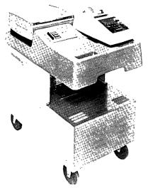
Power source is a standard 12volt, storage battery. Under normal operating conditions, power can be generated for a full working day; connection to an ordinary wall outlet fully recharges the battery overnight.
