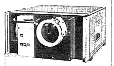
HP 2758A Tape Reader Reroller. Tapes are read photoelectrically, character by character. Model 2758A reads standard one-inch, eightlevel code tape, made of any material with less than 60% transmissivity. Tapes can be intermixed without any adjustments. The only restriction is that metal mylar tapes can't be used in the canister; hence can not be rerolled. The reroller has a tape capacity of 250 feet. (For more information, circle #59 on the Reader Service Card.)
