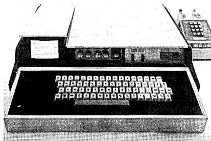
To operate the terminal, the user simply plugs it into an ordinary outlet, folds out the keyboard, pops up the screen, inserts an ordinary telephone into the built-in acoustic coupler and dials his computing center or service bureau. (For more information, circle #70 on the Reader Service Card)
