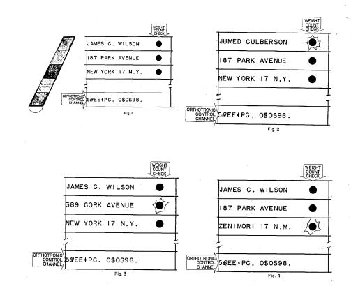
The attached diagrams illustrate the power of Orthotronic Control to correct or restore recorded information that has become garbled or lost within the data processing system.
