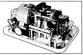
small and have a large margin available to increase reliability. A pushbutton is incorporated underneath the unit to cock the punches when a machine is first put into service or after repair since it is advisable to store a machine with the punches in the released position.
