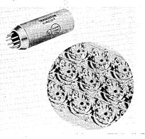
the recommended 1 inch spacing, the total space required is 1 square inch per case or 2.18 cubic inches per case. Cases may contain more than one circuit, are not potted, and can be opened without special tools for repairs if necessary. No non-standard punching or expensive connectors are required. For information write EN-GINEERED ELECTRONICS CO., P. O. Box 659, Santa Ana, California.
