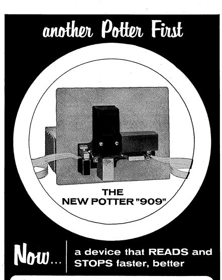
The compact '909' Perforated Tape Strip Reader now makes it possible to process information from perforated tape into digital data computer systems at high speed and low cost. Simple to operate by clerical personnel, the '909' is completely transistorized, and will give maximum performance with complete reliability.
