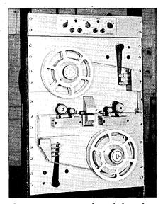
characters per second, with less than 5 milliseconds start or stop time. At 300 characters per second it stops in the space following the stop character. For 750 character per second operation, a two character stop space is recommended. All standard 5, 6, 7 or 8 level tapes (plus sprocket hole) are handled and 11/16 in.,  $\frac{7}{8}$  in. or 1 in. wide tapes can be used interchangeably. Other characteristics include complete remote control of forward,
