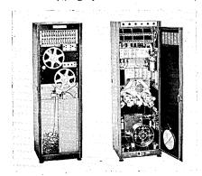
stores and reproduces analog or digital data. Two independent capstan drives with high speed start-stop times of less than 2 milliseconds, permit tape to operate in either direction at speeds from 60 ips to 150 ips. Tape widths from  $\frac{1}{4}$  to 2 in., storage bins for 3,000 in. of tape, modular construction and moderate power dissipation are listed as outstanding features. For information write D. G. C. HARE CO., 30 Burtis Ave., New Canaan, Connecticut or use reader card.
