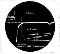
order of 50 times faster than other available computer diodes, according to the manufacturer. New manufacturing techniques have resulted in a stored charge (after a 10 ma forward current) smaller than that of a 3 micro-microfarad capacitor at 6 volts. Another diode, the S555G, is specified at 6 milli-microseconds and offers better dc characteristics. For information write TRANSITRON ELEC-TRONIC CORP., Wakefield, Massachusetts or use reader service card.
