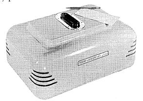
control. It would be possible to use both positions for information only but in this case some additional clamping control would need to be provided. A further switch at the top of the unit indicates that a card has entered. The switching is so arranged that the sequence-top switch followed by bottom sensing switch-must be observed before the card is clamped. This ensures that a card is removed completely before operation is started.
