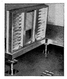
Reinforced, stringer-free aluminum panels permit total access to sub-floor; allow cut-outs anywhere on the panel, even after installation, while retaining maximum strength, minimum deflection. Adjustable pedestals assure perfectly level floor.
