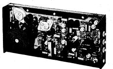
100 meg input impedance, gain accuracies to  $\pm$  .002%, linearity at .005% minimum and less than .01% noise peak-to-peak, from any source. Each unit is completely self powered. For information write PACKARD BELL COMPUTER CORP., 1905 Armacost Ave., Los Angeles 64, Calif. Circle 202 on Reader Service Card.
