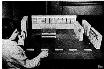
Top—Exhibited at AUTO MATH 59 was this HIPAC 101, manufactured by Hitachi Ltd. of Tokyo. HIPAC stands for HItachi Parametron Automatic Computer. It is a binary, fixed point machine.
