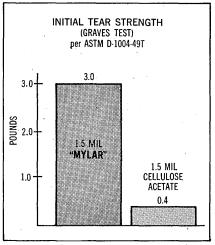
Reduced breakage from edge nicks. Chart 2 shows the initial tear strength of "Mylar" is over seven times that of acetate. "Mylar" resists edge nicking and retards growth of tears if nicking occurs. Since most tape breaks start as edge nicks, you'll have less tape breakage and loss of valuable information with "Mylar".
