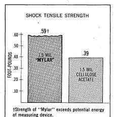
Less breakage from shock. Chart 1 compares shock tensile strength of "Mylar" with that of cellulose acetate. The strength of "Mylar" actually exceeds the range of the measuring device, while acetate failed at 0.39 foot-pounds. With "Mylar" you'll have less tape breakage from high-shock loading sometimes created by operating conditions. And, "Mylar" does not lose its strength with age, repeated playbacks or storage, because it has no plasticizer to dry out.
