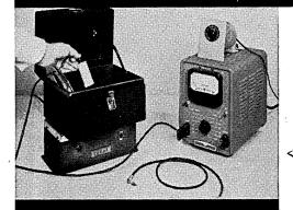
Test factually demonstrates shielding effectiveness of Netic alloy material and enclosure design. Instrumentation used: magnetic field radiating source. AC vacuum tube voltmeter, Variac. pickup probe and Netic Tape Data Preserver. For complete test details and results, request Data Sheet 142.
