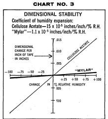
Fewer weak or garbled signals. Chart 3 shows dimensional change in "Mylar" with temperature or humidity change is negligible compared with that of cellulose acetate. This exceptional stability prevents tape shrinking, swelling or cupping that could result in shifting of tracks or loss of contact with the recording or playback head. Possibility of signal dropout or garbled or weak signals is minimized, and reliability of recorded data is improved.
