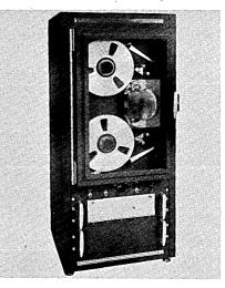
servos. Uni- or bi-directional fast stopstart modes are possible for all types of programs. Both fast forward and fast reverse modes are servo controlled for constant tape tension, thus assuring gentle tape handling. SHEPHERD IN-DUSTRIES, INC., 103 Park Ave., Nutley 10, N.J. For information: CIRCLE 208 ON READER CARD
