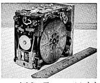
insure reliability. The tape unit includes a tape remaining indicator that transmits its information to the ground along with its communication data. All electronics use solid-state components and include record and reproduce amplifiers and a power supply which converts dc to ac for the drive motor and regulates the dc supply. CONSOLI-DATED ELECTRODYNAMICS CORP., 360 Sierra Madre Villa, Pasadena, Calif. For information:
