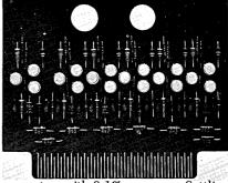
converter, with 0.1% accuracy. Settling time for a full scale voltage change, 10 volts, is 2 usec. The converter can be driven by stroke gates and flip-flops. Output impedance of the converter is 2250 ohms. ABACUS, INC., 3040 Overland Ave., Los Angeles 34, Calif. For information:
