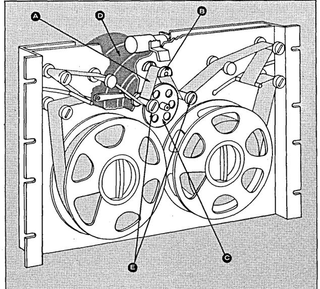
Line by line cycle: movement of tape (A) over read head (B) is controlled by drive capstan (C)—attached directly to shaft of PMI printed motor\* (D); spring-loaded rollers (E) hold tape gently against capstan, keeping tape movement in exact accord with capstan rotation; advance command pulse accelerates motor, capstan, and tape; as read head detects next sprocket hole, a reverse pulse to motor halts capstan and tape with next character perfectly aligned in read head.
