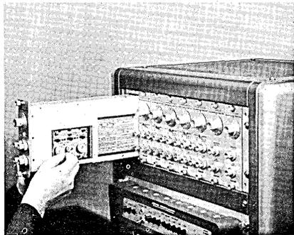
oscillograph which has 12 chart speeds from 0.05 mm/sec. to 200 mm/sec. Approximate price, including pre-amplifiers, is \$13,000. BRUSH INSTRUMENTS, 37th and Perkins, Cleveland 14, Ohio. For information:
