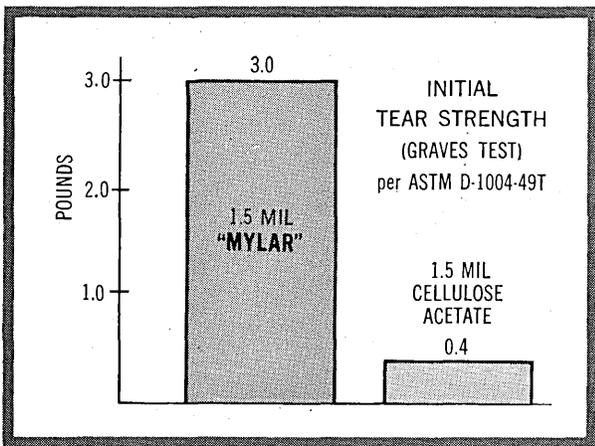
Every minute of downtime costs you dollars. That's why the reliability of your magnetic tape is so important. Tapes of Mylar\*, resist breaking from sudden starts and stops since they have high shock-tensile strength . . . and they have 7 times the initial tear strength of acetate tapes.
