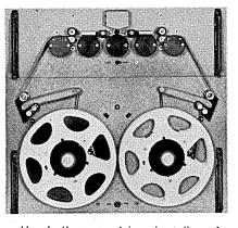
Here's the newest in a long line of superior Rheem punched-tape readers and spoolers — the RR-300MB Bidirectional Tape Reader coupled with the RS-300M Tape Spooler. Reader features include the ability to read 8 level tape plus sprocket hole at 300 characters per second continuously, and stop on character. Reading capabilities also include 100 characters per second normally in asynchronous or line-at-a-time mode, and up to 200 characters per second in special applications.
