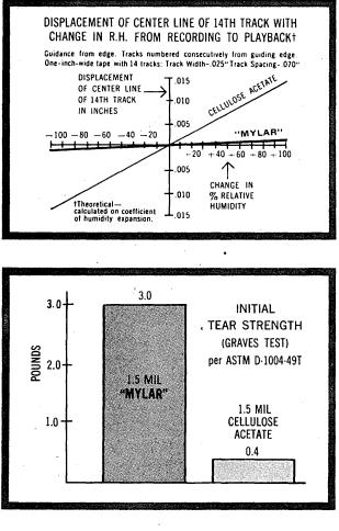
An unreliable tape can shrink or swell—cause garbled signals because the tape tracks shift laterally away from the recording and playback heads. With tapes of dimensionally stable "Mylar"\* polyester film you get accurate results . . . valuable programming time is saved.
