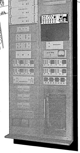
Fabri-Tek memory system installed in U.S. National Bureau of Standards Digital Correlator for Jicamarca Radar Observatory near Lima, Peru.
