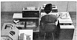
Each 1050 installation may include from one to six input/output devices, including printers, card reader, card punch, paper tape units, keyboard. These easily connected units may be used for local data handling as well as long-distance communication.
