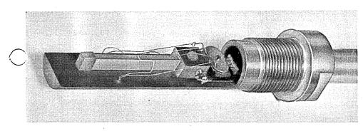
An elegant, but tiny refrigerator, utilizing the Nernst-Ettingshausen effect, has been demonstrated in the Solid State Physics Laboratories at Lockheed Missiles & Space Company. This type of cooling is applicable below 200° Kelvin, where thermoelectric cooling is no longer efficient. It shows particular promise for space application because of the reliability inherent in its all-solid state construction.
