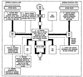
ence of the start bit and code bits. The code bits are assembled into five-bit Baudot characters and packed three characters per computer word. These words are then stored as message segments in bins (typically 32 words) in main core storage. (The assignment of bin locations is handled by a closed subroutine called the available bin program, which allots available bins to all requesting routines. Depending on the system, up to 512 bins are reserved for this function).
