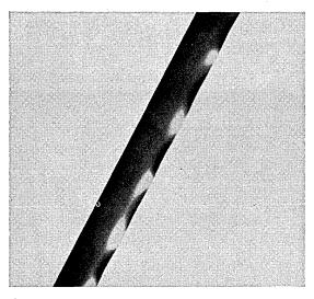
**Complaint.** Wavy edge caused by improper slitting. **Solution.** Specially designed Memorex slitters and microscopic edge inspection of every reel prevent wavy edges. Fifty-one other quality control checks (many performed only by Memorex) guarantee every Memorex reel pre-test perfect.
