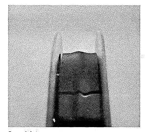
**Complaint.** Semi-permanent ridging and loss of contact caused by microscopic scratches produced in manufacturing or use.
