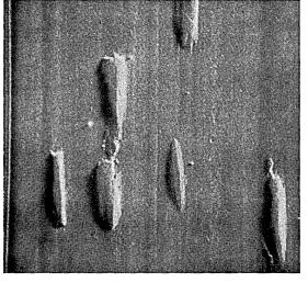
**Complaint.** Dropout-causing clumps of redeposited coating (50X magnification).
