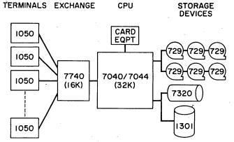
essing; an IBM 1301 disc storage for storing inactive user programs in the library; and IBM 729 magnetic tape units for on-line recording of operating statistics and offline assignment to conventional operating system functions.
