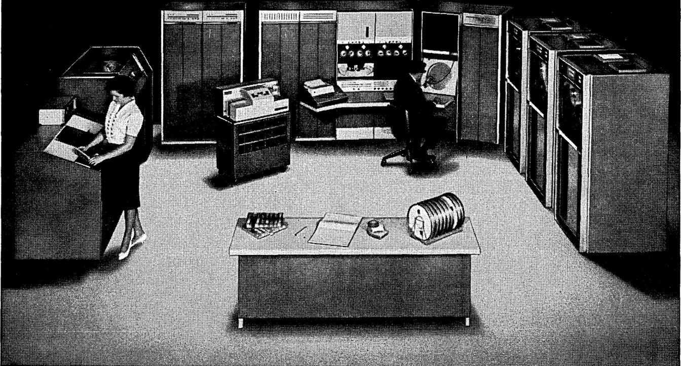
By *power*, we mean a 2-microsecond cycle time, ability to directly address 262,144 words of memory, a 36-bit word, 7-channel priority interrupt, 363 instructions, FORTRAN, an I-O system for 128 devices... and much more.
