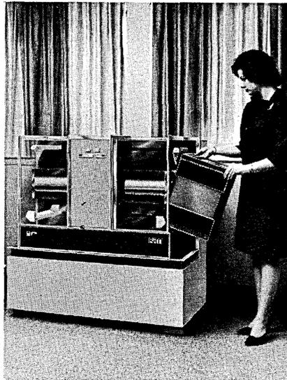
transfer rate is 600,000 bps. The single-capstan transport, Model SC-1150, operates bidirectionally up to 150 ips at 800 bpi with no program restrictions, said to be a first in transports. Other features are 7- or 9-channel operation for IBM 360 and ASCII compatibility; a tape path with no rollers or air guides; and a read/write head which is retractable during rewind and stop.
