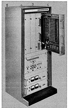
If you don't want to buy the fastest megabit memory system complete, we suggest that you build it yourself. Because of the unique modular construction of Nanomemory you can buy the complete memory system, the digitized stack only, or just the core stack assembly. In each case you get nanosecond cycle times, 2½ D organization, and highly competitive prices.
