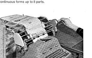
Get continuous production from typewriters or bookkeeping machines. Moore Flexible Formaliner permits use of continuous forms in typing; Vertical Spacer skips forms past non-write areas.
