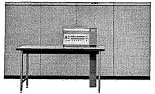
SDS 920 has the same memory capacity and priority interrupt as the 925. One standard and one buffered
