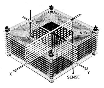
The memory designer must pay for delay in two ways. In a coincidentcurrent memory, the X and Y currents must travel through the entire stack to select all cores. Breaking up the stack into smaller modules increases circuitry costs. Also, the sense line has a definite length which contributes to the delay.
