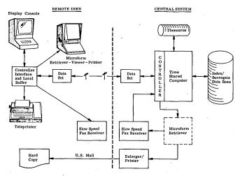
Fig. 2. Remote User/System Communication
