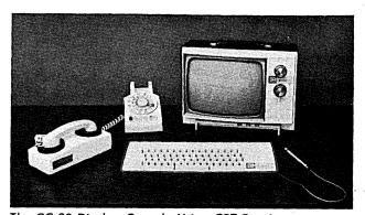
The CC-30 Display Console Using CRT Receiver.
