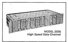
The RFL Model 2056 operates at any speed up to 2400 bits per second on a non-synchronous basis on standard bands, and much higher, with wider bands. It uses frequency shift keying and special techniques for reducing fortuitous distortion or jitter and is relatively unaffected by variations in signal and high noise levels.
