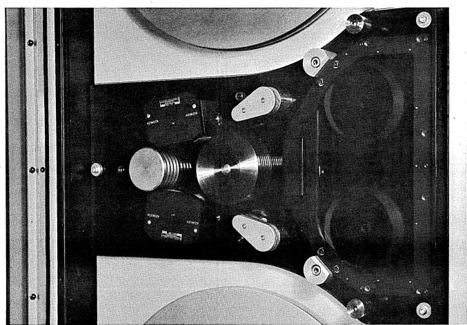
DUAL INERTIA DRIVE, INERTIA DISENGAGED
