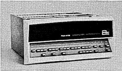
dex register, conditional jumps, parallel processing, block I/O, and three priority interrupts. Available peripherals include Teletype, mag and paper tape, disc, and modems. The company says the unit undergoes 16K hours of test operation before it is marketed to ensure trouble-free functioning. The price is \$11,900. COMPUTER AUTOMATION, INC., Newport Beach, Calif. For information:
