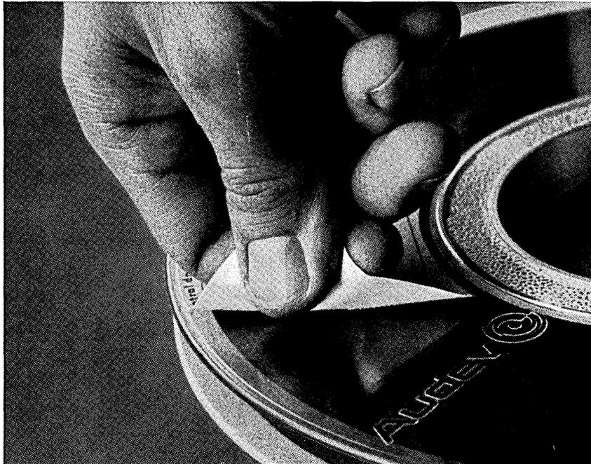
With proper handling, computer tapes can be "scratched" and reused almost indefinitely. However, careless removal of previous labels can
