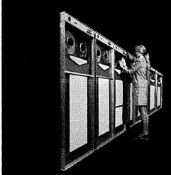
AMPEX TM-1624, TM-1629 75/112.5 ips; 300 ips rewind; 180kHz transfer rate; 3 msec start/stop. AMPEX TMZ 10-24 ips; 150 ips rewind; 19kHz transfer rate; 18 msec start/stop; all electronics included.
