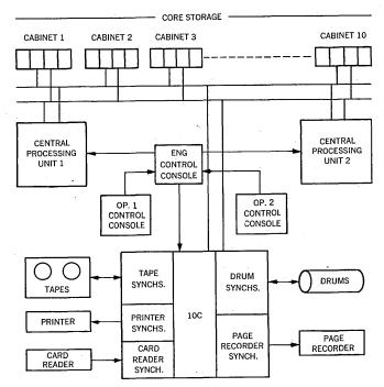
Fig. 1—Block Diagram of a LARC System
