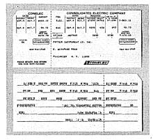
card preparation. A magnetic mark card reader reads the six-line cards produced both manually and automatically at 300 cards per minute. The hole-free cards provide an effective and convenient turnaround document which is especially suited for utility billing and similar applications.
