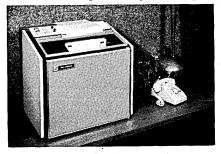
cessing terminals and small computer systems. It will print at up to 1050 lpm, 80 columns wide, with a 64-character alphanumeric set. The 4800 utilizes either fan-fold paper with sprocket feed, printing up to six copies, or friction-feed paper rolls. A unique feature is the ability to remove and re-
