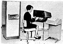
central processor in either parallel or serial mode at transfer rates from 300 to 4800 bps. An IBM-compatible interface adaptor is available; interfaces for other computer systems are available on request.
