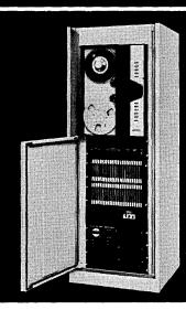
AMPEX BTM (Buffered Tape Memory) 45-150 ips; 500,000 bytes/ sec short term transfer; 102,000 bytes/sec long term transfer; 556/800 bpi density.
