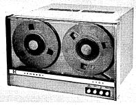
capstan drive is 15 ms, and slew or rewind speed is approximately 120 ips. The small reels used accommodate 1,200 feet of tape. Read and write electronics are not included in the price, but read, write, read/write, or read-after-write controls are available. Internal parity generation is standard, as is ccrc in the nine-track versions. Control electronics are included in the \$2.6K offering. KENNEDY CO., Altadena, Calif. For information:
