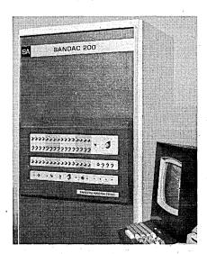
ented instruction set with 65 basic commands; 15 hardware index registers with double indexing; and communications supervisory program and subroutine library. Memory parity and overwrite protection, real-time clock, dynamic core allocation, remote pro-
