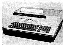
dinary telephone lines, the terminal provides 96-character full usascii capabilities. Its additional 32 characters include symbols and lower case alphabet. Included as integral components are a keyboard; a 10, 15 or 30 cps (operator selectable) thermal page printer; solid-state control logic; built-in telephone coupler and interface; and a universal interface for peripheral accessories. All this and the carrying case weigh less than 30 pounds.
