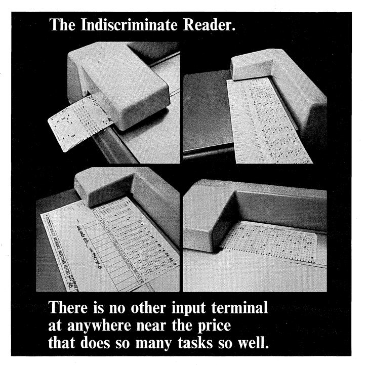
The Motorola Indiscriminate Reader will read ordinary pencil-marked data, keypunched data, preprinted data. In any combination. In any column-spacing format.
