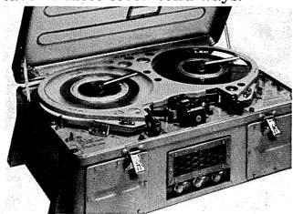
Save weight. At a compact 36 lbs., the incremental ADR 445 is about one-fifth (or less) the weight of other airborne data recorders.
