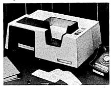
mand rate of 300 80-column cards per minute with every card under computer control, with the ability to pick on demand at any rate up to the 300 card-per-minute maximum. The use of TTL logic, solid-state plug-in modules and convenient test points is said to simplify maintenance. The SR-300 measures 20" wide by 15" high by 22" deep and weighs approximately 70 pounds.
