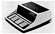
direct and indirect store and recall of data registers enable it to invert a matrix up to 10 X 10. The unit has its mag tape for some I/O, and augments this with provisions for typewriter output. A "learning" mode enables step-by-step program use or checkout. At \$4,900, the price approaches that of a cpu, too. WANG LABORATORIES, INC., Tewksbury, Mass. For information:
