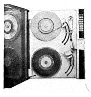
6000 and 6600 oem tape transports. Since the 6000 series consists of synchronous read-only units, their primary application areas will be for use in computer output microfilmers, offline printing and plotting, and photo typesetting. The 6600s are read/write units. Error recovery features and a choice of any two densities are
