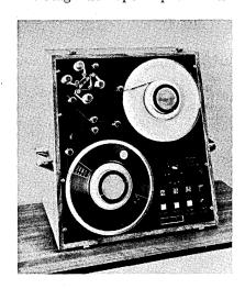
rended to be economic for tape libraries of 2,000 or more reels. It not only inspects for dropouts, but removes dirt and oxide particles from the tape surface. Cleaning is repeated until dropouts are reduced to an acceptable level. Threshold is adjustable to 50, 60, or 70% of normal signal strength. Both 800 and 1600 bpi tapes are handled, and a model is
