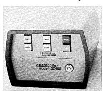
trillion unique code formats are possible in this version, which can operate over dial-up and dedicated phone lines, and even microwave links. The speed of the DC-110 is given as 100,000 baud through tty or Rs-232 interface. Prices for the DC-108 and DC-110 are \$2950 each—and don't forget that you need at least two of them. For information: CIRCLE 212 ON READER CARD
