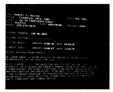
**Two-level video intensity.** Useful for form fillout. Computer-derived protected data is lower intensity; operator-entered data is brighter. **Selective scrolling** at any line when under program control; automatically at line 1, unless otherwise directed.
