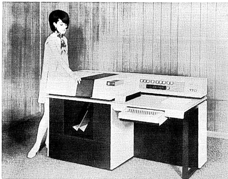
is 100 cps. Spacing is 3 lines/inch for double space, 4½ for one-and-a-half space, and 6 lines/inch for single spacing (upper case only). Margins should be at least one-half inch on either side. Any character that cannot be recognized is displayed to the operator on an optical display—using no electronics, to further reduce cost—for correction via input from an alphanumeric keyboard.
