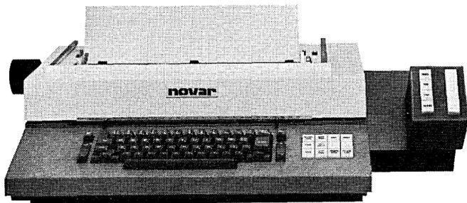
This terminal can be equipped to "carry on" automatically — at any hour and without an operator. It can transmit data, or receive data at high speed from a computer and print at night to be ready for the next day. Ask about Unattended Operation capability.
