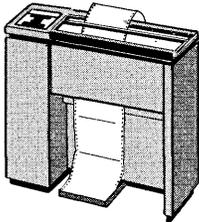
**DT-8280 Data Terminal.** A remote print station that operates at speeds in excess of 4800 baud—available in 132-column (above) or 80-column models. Comprehensive formatting including data compression. Replaces teletypes or IBM 2780. Prints up to 1110 lpm. Handles up to 6-part paper.
