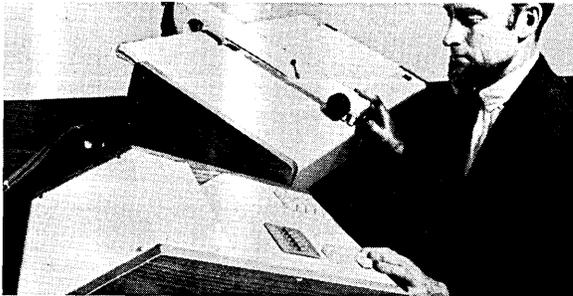
Many companies are looking to Electronic Systems Limited, Downsview, Ontario, for the equipment they know will make their job easier—like this Model 11 Digitizer which collects graphic information and converts it directly to computer-compatible input. The Model 11 is fast, simple to operate and inexpensive, yet accurate to .01 inches.
