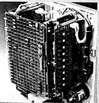
Magnetic Tape Formatters, embedded or stand-alone models, provide all necessary logic for reading and writing PE or NRZI formats on both 7-track and 9-track tapes. The space and cost saving microprogrammed embedded formatter is contained on a single multi-layer PWB within the transport.
