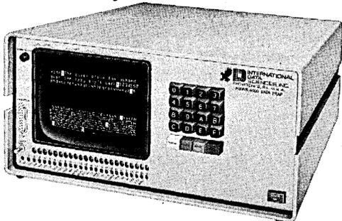
The Hawk 4000. It's IDS's new Data Trap with a microprocessor that lets you diagnose data communications problems quickly. The Hawk is interactive. It can monitor, transmit, and receive data between a modem and terminal on a big 9", 512 character screen. And, 2000 characters can be trapped and stored for later recall and study.
