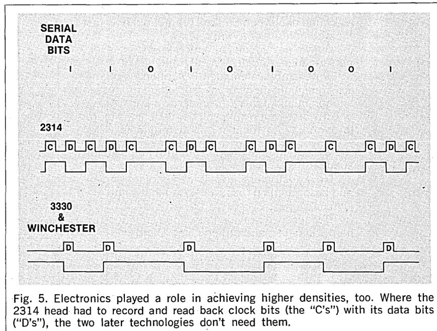
Fig. 5. Electronics played a role in achieving higher densities, too. Where the 2314 head had to record and read back clock bits (the “C’s”), the two later technologies don’t need them.
