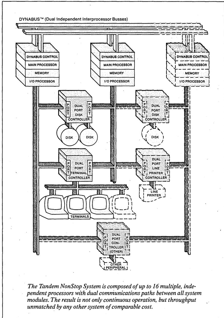
*The Tandem NonStop System is composed of up to 16 multiple, independent processors with dual communications paths between all system modules. The result is not only continuous operation, but throughput unmatched by any other system of comparable cost.*
