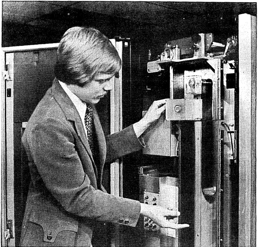
Both the IBM 3850 and Control Data 38500 mass memory systems are basically tape libraries. Although each has mechanisms for storing and retrieving cartridges, within the cartridges there is 3-inch wide magnetic tape. As shown in the CDC photo above, the tape is removed from the cartridges and then read or written in a conventional manner.
