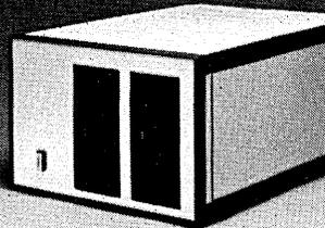
Flexible Disk Drive Systems for interface to PDP-11 and NOVA computers are available in one to four drive configurations for low cost data storage in IBM compatible format.
