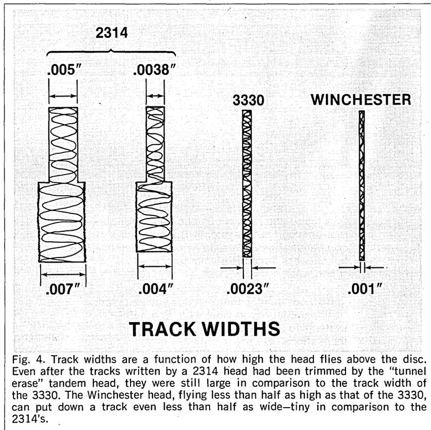
Fig. 4. Track widths are a function of how high the head flies above the disc. Even after the tracks written by a 2314 head had been trimmed by the “tunnel erase” tandem head, they were still large in comparison to the track width of the 3330. The Winchester head, flying less than half as high as that of the 3330, can put down a track even less than half as wide—tiny in comparison to the 2314’s.
