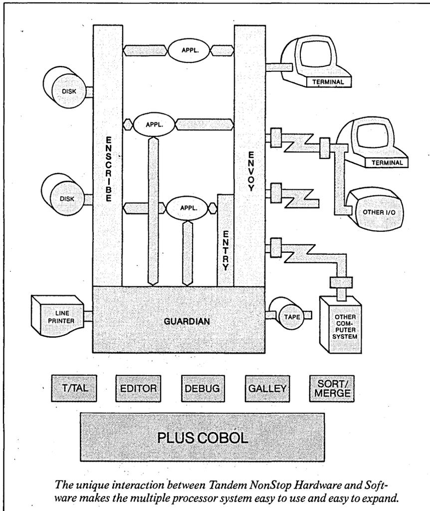
beginning of the program to set the NonStop mode. From then on, CHECKPOINT controls passing information to the backup process at critical points. CHECKPOINTS occur automatically at any OPEN or CLOSE after the backup is established. These two simple instructions eliminate the downtime, restart, and revalidation which plague any user without the Tandem NonStop capability.
