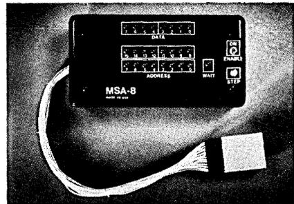
provides single step, hardware breakpoint, and oscilloscope trigger capabilities. LED's display the status of the data and address lines. The MSA-8 sells for \$249. COMPUTER SYSTEMS DYNAMICS, Salt Lake City, Utah.
