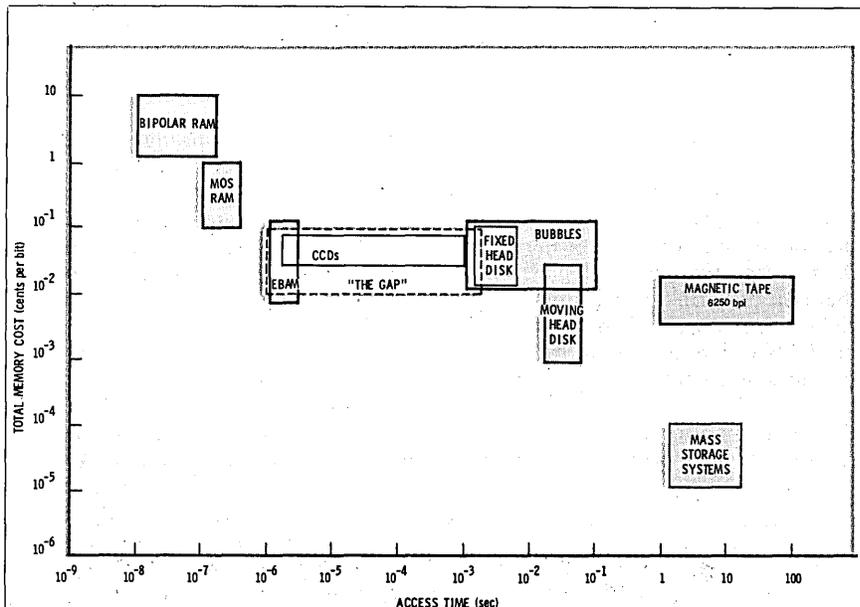
Fig. 2. Moving head discs are cheap enough, but not fast enough to close the gap; CCDs are almost fast enough but not cheap enough. So the gap will exist for some time yet.
