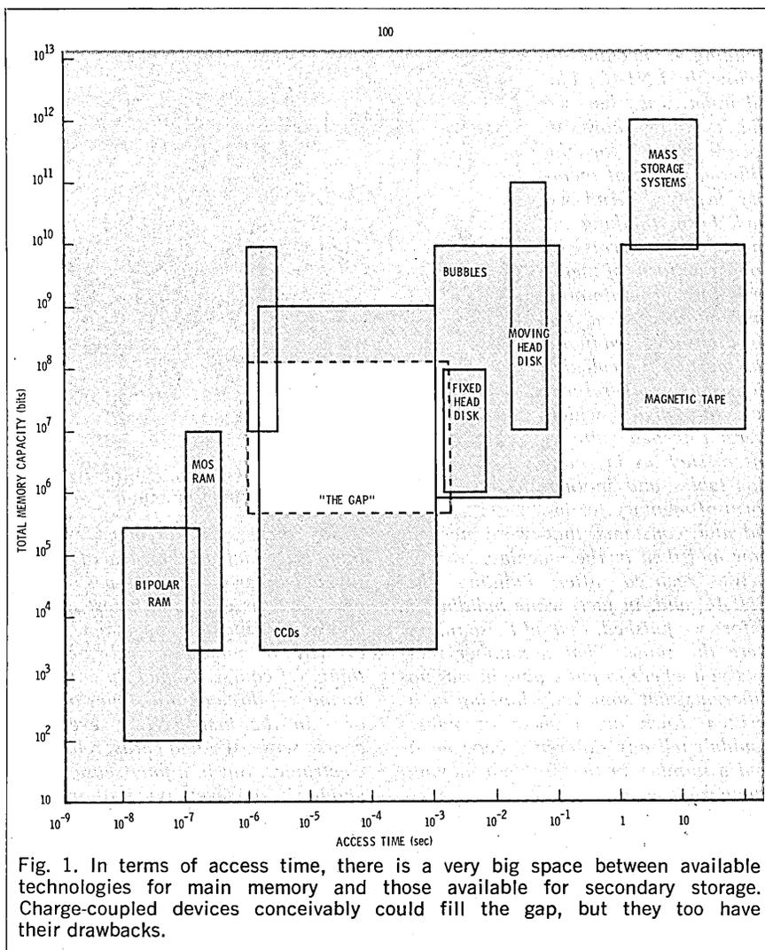
Fig. 1. In terms of access time, there is a very big space between available technologies for main memory and those available for secondary storage. Charge-coupled devices conceivably could fill the gap, but they too have their drawbacks.
