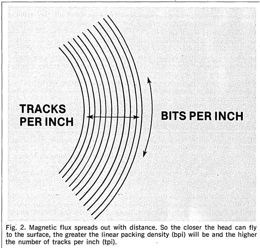
Fig. 2. Magnetic flux spreads out with distance. So the closer the head can fly to the surface, the greater the linear packing density (bpi) will be and the higher the number of tracks per inch (tpi).
