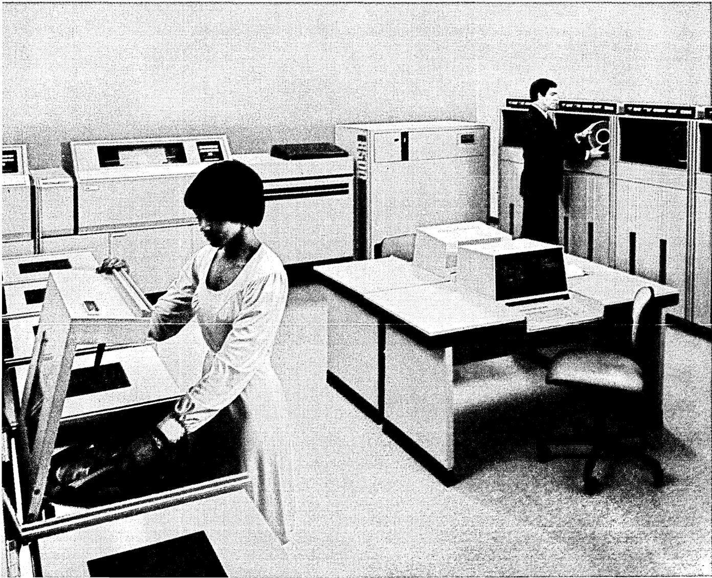
It uses multilevel pipeline processing. As each program instruction is executed, the next three instructions are simultaneously advanced toward execution to provide greater efficiency.
