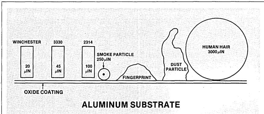
Fig. 3. The reason for controlling the disc environment, and for sealing the packs, becomes apparent when we realize that a smoke particle roughly 250 millionths of an inch in diameter simply won't fit between the read/write head and the disc surface. To a flying head, a fingerprint looks like a mountain. In comparison to these obstacles, the major differences in the flying heights of the three kinds of heads does not show up in this scale.
