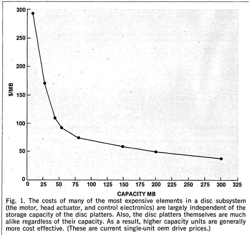
Fig. 1. The costs of many of the most expensive elements in a disc subsystem (the motor, head actuator, and control electronics) are largely independent of the storage capacity of the disc platters. Also, the disc platters themselves are much alike regardless of their capacity. As a result, higher capacity units are generally more cost effective. (These are current single-unit oem drive prices.)
