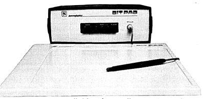
Bit Pad is the low-cost digitizer for small computer systems. Better than a joystick or keyboard for entering graphic information, it converts any point on a page, any distance into its digital equivalents. It's also a menu for data entry. You assign a value or an instruction to any location on the pad. At the touch of a stylus, it's entered into your system.
