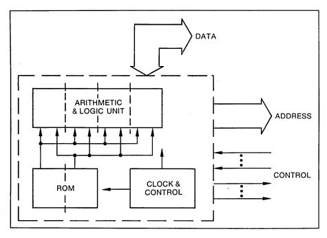
Fig. 2. The microprocessor in a bit-slice microcomputer, as with any other central processor, must have arithmetic and holding registers, the program counter, instruction decoding logic, and sequencing logic. But it also must have a ROM associated with it to store the microprograms used for executing its instructions.
