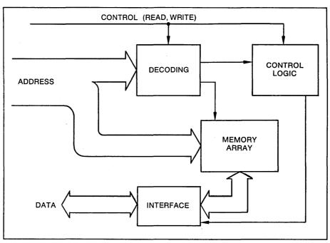
Fig. 3. This illustrates how a typical microcomputer memory system might be organized. Certain bits of the address field are decoded to select elements of the memory array while lower-order bits select words within those elements. Data is read out to or written into those places from the data bus. The control logic might include latches for holding input or output data, refresh circuitry if the memory is dynamic, and so on.
