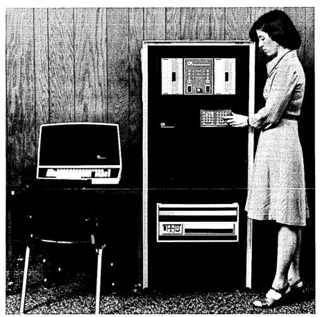
Computer Automation's Naked Mini 4 illustrates how broad the range of minisystem packages can be. Available in stripped form (with 4K of memory, power supply, chassis, and console) for \$995, it also can be delivered in configurations like the one above (with hard disc, soft disc, crt, extended memory, etc.). In fact, "typical" systems can run 10 to 15 times as much.
