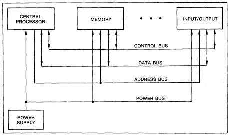
Fig. 5. In modern microcomputers, the cpu, memory, and I/0 subsystems are connected by busses for control signals, data, addresses, and power.
