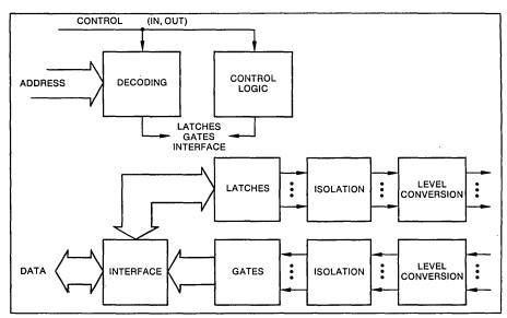
Fig. 4. This illustrates how an I/O subsystem might be organized. Addresses are decoded to select specific ports—which will be sets of logic gates for outputs to the data bus or sets of latches for inputs to the memory.
