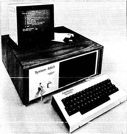
The System 8813, part of PolyMorphic's System 88 line, features BASIC and disc operating system, and exemplifies the microcomputer systems' approach to business applications.
