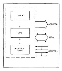
Fig 1. These are the main components of the central processor in a microcomputer. The clock steps the logic from one state to another and synchronizes data transfers. Control logic manages data transfers. In some cases, interrupt logic is also included.
