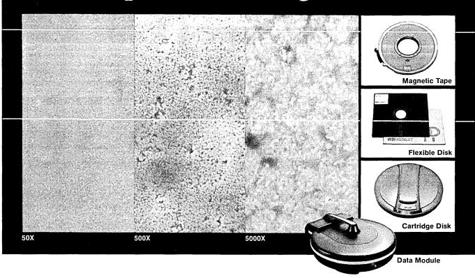
A close look at a section of disk through a scanning electron microscope taken at 50X, 500X and 5000X shows the magnetic oxide coating of the surface. The quality of the surface is of the utmost concern, because of the increasing requirement for higher densities.
