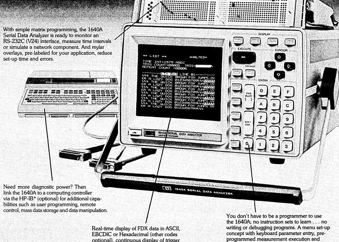
optional), continuous display of trigger specifications, and clear display of measurement results all add up to a convenient presentation of "what's happening" in your computer network.
