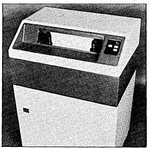
swing-out yoke and in-line paper tractors simplify forms loading, and 69 interchangeable type bands, covering 22 languages, are available. A 300 lpm model sells for \$5,995, a 600 lpm model is \$8,995, and a 900 lpm unit goes for \$12,995. FOR DATA CIRCLE 412 ON READER CARD
