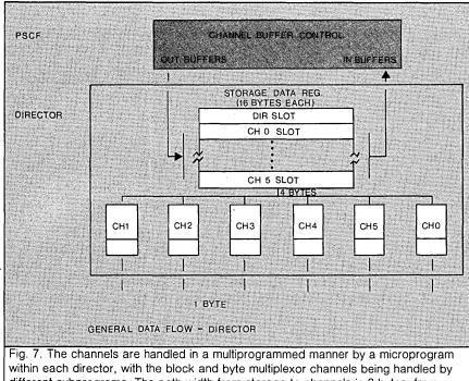
within each director, with the block and byte multiplexor channels being handled by different subprograms. The path width from storage to channels is 8 bytes, from channels to storage 4 bytes, from the director's registers to channels 4 bytes, and those to the outside world are 1 byte (although the first block multiplexor of any group may have a 2-byte wide path).
