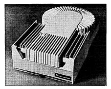
controller. The D160's sealed disk modules contain two platters for 60MB capacity, three platters for 90MB, or four platters for the maximum 120MB; the modules also contain four, six, or eight heads, respectively. Servo data, interlaced in each track, are used for head positioning. Oem pricing, for annual quantities of 100, runs \$3,085, \$3,355, and \$3,625 for 60мв, 90мв, and 120MB versions, respectively. FOR DATA CIRCLE 404 ON READER CARD
