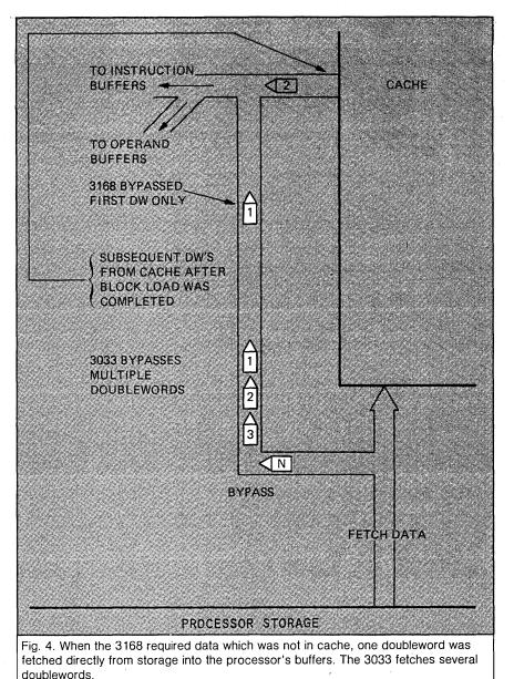
operand data, and, in particular, the move character operation (MVC) can prefetch up to five doublewords of source operand. (The 3168 operand prefetch is limited to one doubleword per operand, unaligned.)
