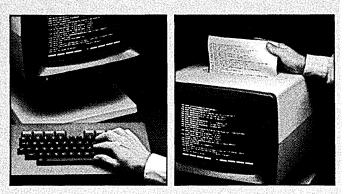
Try this on your favorite CRT! With the 2621P, you just hit a key and in seconds you have hard copy of your CRT display. The built-in thermal printer prints upper and lower case at up to 120 cps.
