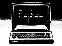
A full-featured CRT, plug-compatible with IBM 3275, to display and communicate your data at 4800 bps over dial-up lines and 9600 bps over dedicated lines.
