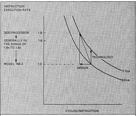
Fig. 1. A processor's internal performance is a funciton of technology and machine design. Thus the performance improvement of the 3033 over that of the 3168 is due partially to technology (reduing the cycle time from 80nsec to 57nsec leads to an increase in instruction execution rate of about 40%) and partially to design improvements which act to reduce the number of cycles per instruction.
