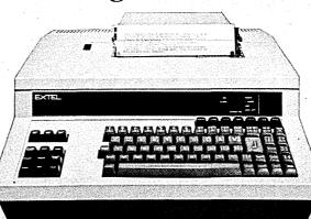
Extel's new B31 communications terminal will automatically relay switching protocol, dialing and addressing sequences. This is true for the TWX or DDD networks, or message/packet systems accessed by public or private networks.
