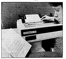
ASCII set. Reverse channel, XON/XOFF, and Data Terminal Ready protocols are switch selectable, as are parity, number of stop bits, and data rates ranging from 110bps to 9600bps; the unit has a standard buffer size of 256 bytes (2кв is optional). The 704 has an RS232 interface. Available in three models, the 704 is priced from \$2,350 to \$2,665 (end user pricing).
