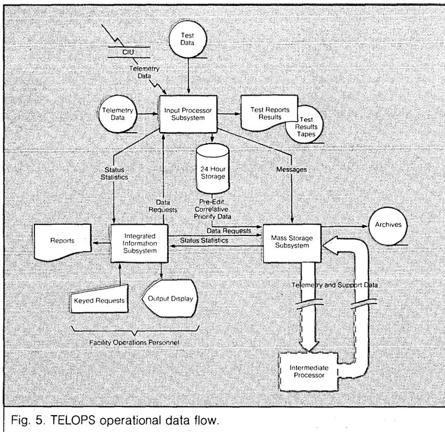
Fig. 5. TELOPS operational data flow.
