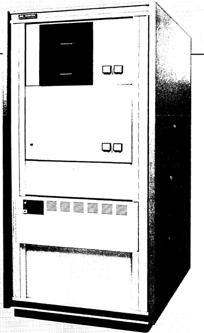
Series, the C3-B. Its specifications are the same as those of the C3-C. However, the C3-B offers a 74 Megabyte Winchester drive.
