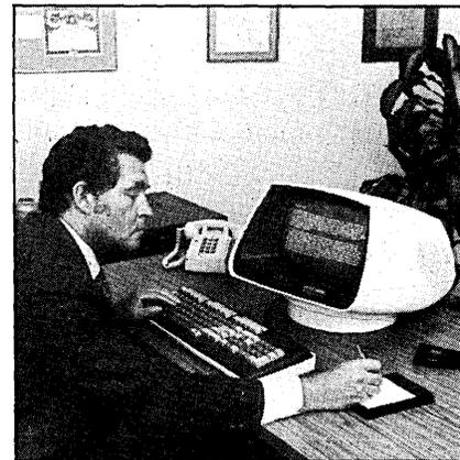
vendor's computers, the terminals display the upper- and lower-case ASCII characters formed in a 7 x 11 dot matrix cell; the display screen has a capacity of 24 lines of 80 characters. Both terminals have typewriter-style keyboards and 14-key numeric clusters; additionally, the D200 has a 12-key screen management keypad, and a 15-key function keypad. A subset of D200 func-
