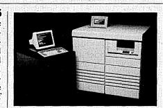
ing up to 224 users, the H 1200 utilizes 100K ECL (emitter coupled logic) and gate array circuits. The H 1200 software is compatible with the rest of the H Series. Prices for the HCX-7 start at \$225,000. The H 1200 starts at \$249,000. HARRIS CORP., Computer Systems Division, Fort Lauderdale, Fla. **FOR DATA CIRCLE 300 ON READER CARD**  over the format and content of reports.
