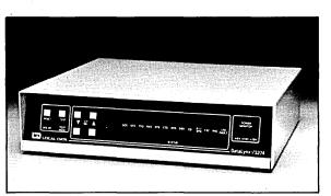
DataLynx/3274 connects 1 to 9 async CRTs and printers to a 3270 multipoint network, SNA or BSC.
