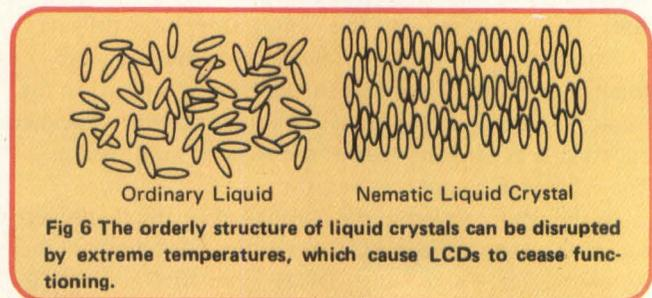
Fig 6 The orderly structure of liquid crystals can be disrupted by extreme temperatures, which cause LCDs to cease functioning.
