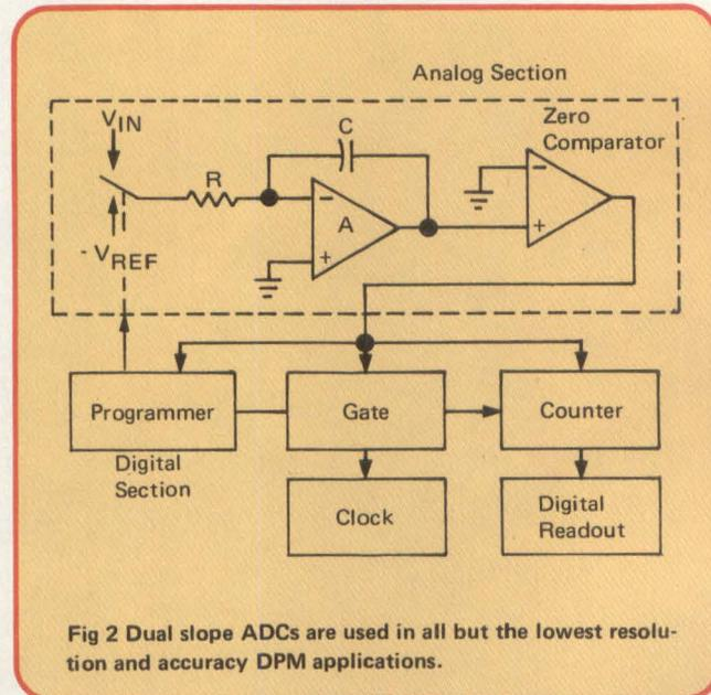
Fig 2 Dual slope ADCs are used in all but the lowest resolution and accuracy DPM applications.
