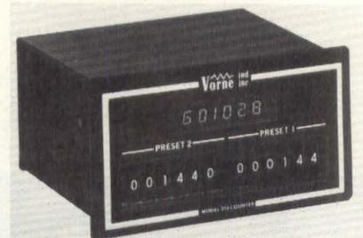
Model 215-Dual, which mounts in panels up to  $\frac{1}{2}$ " thick and measures 2  $\frac{5}{8}$ " H x 3  $\frac{1}{8}$ " W x 4  $\frac{1}{4}$ " D. It operates from 115 Vac. Price: \$234. Vorne Industries, Inc., 5023 West Belmont, Chicago, IL 60641. (312) 725-3077. **Circle 129**
