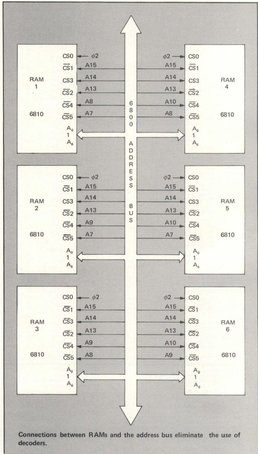
pins for RAM selection optimizes decoding. A RAM selection field n bits long should consist of m 0's and (n-m) 1's, where m is the number of negative CS inputs reserved on each IC. The field can be arranged in  $n!/m!(n-m)!$
