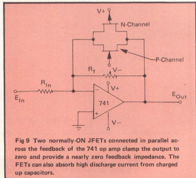
Fig 9 Two normally-ON JFETs connected in parallel across the feedback of the 741 op amp clamp the output to zero and provide a nearly zero feedback impedance. The FETs can also absorb high discharge current from charged up capacitors.
