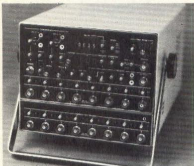
cursor. The 50DI6 package measures 6 $\frac{3}{4}$ " x 8 $\frac{1}{2}$ " x 14", and weighs 18 pounds. Price: \$4,558. A data formatter option makes the 50DI6 fully software compatible. BP Instruments, Inc., 10601 S. DeAnza Blvd., Cupertino, CA 95014. (408) 446-4322. **Circle 130**
