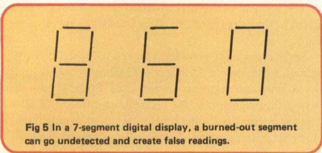
Fig 5 In a 7-segment digital display, a burned-out segment can go undetected and create false readings.
