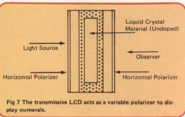
**Fig 7** The transmissive LCD acts as a variable polarizer to display numerals.
