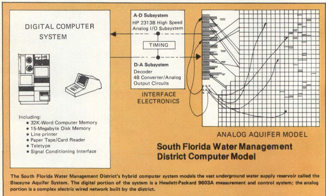
Given historical and current data on water levels, depth of the aquifer and other factors, planners program the model to simulate the effects of increased or decreased rainfall, more pumping, new well-fields, or other changes in land use or the water picture that will affect the future water supply of South Florida.
