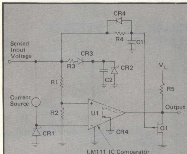
Fig 7 Precise voltage level detector, powered by the sensed potential, contains two principal circuit components, U1 and Q1. U1 is a high gain differential IC comparator, such as LM111, which has an open collector output and is able to operate over a wide range of supply voltage. Q1 is a p-channel JFET with a pinch-off threshold lower than the sensed input,  $V_I$  minus  $V_L$ , that controls the output by clamping it to ground level, until the LM111 has had time to stabilize after power ON.
