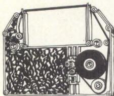
Adding ink with an Accuflo roll maintains print intensity for the life of the ribbon. You get darker characters up to four times as long as with conventional ribbons. Accuflo adds lubricity as it adds ink, so your whole system lasts longer. And if you need specially formulated inks, you can take advantage of our 17 years of experience in ink technology.
