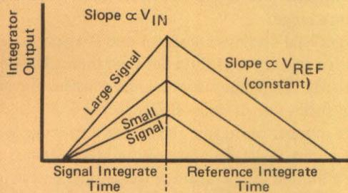
Fig 3 The dual slope conversion technique uses a single clock to govern signal and reference integration periods; thus frequency variations and drift do not affect performance.
