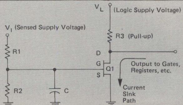
Fig 2 In this basic clear or inhibit circuit, FET switch Q1 turns OFF and ON to provide the required functions.
