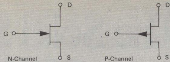
Fig 1 In these normally-ON JFETs, a negative voltage on the gate with respect to the source and drain turns the n-channel device OFF; a positive voltage turns the p-channel device OFF. Most JFETs are symmetrical, since source and drain can be interchanged.
