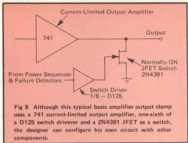
Fig 8 Although this typical basic amplifier output clamp uses a 741 current-limited output amplifier, one-sixth of a D125 switch driver and a 2N4391 JFET as a switch, the designer can configure his own circuit with other components.
