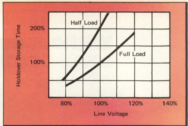
Figure 4: Holdover storage time, the length of time a switcher maintains full output after input power fails, varies: the greater the input voltage and the less load, the longer it is. The relationships are approximately linear.
