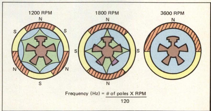
**Figure 3:** Rotor RPMs vary according to power source fluctuations, but exciter head pole-printing speed remains constant. Therefore, even if utility power surges tremendously, jumping rotor speed from 1200 RPM to 1800 RPM, the generator responds by dropping from 6-poles to 4-poles, and output frequency remains 60 Hz.
