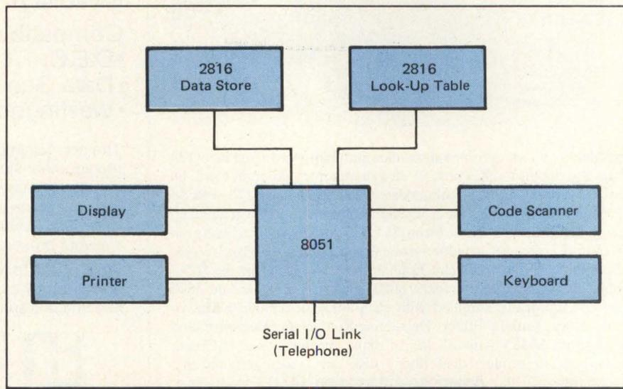
**Figure 1: Point Of Sale (POS) terminal with EEPROMs, permits remote changes of terminal constants.**
