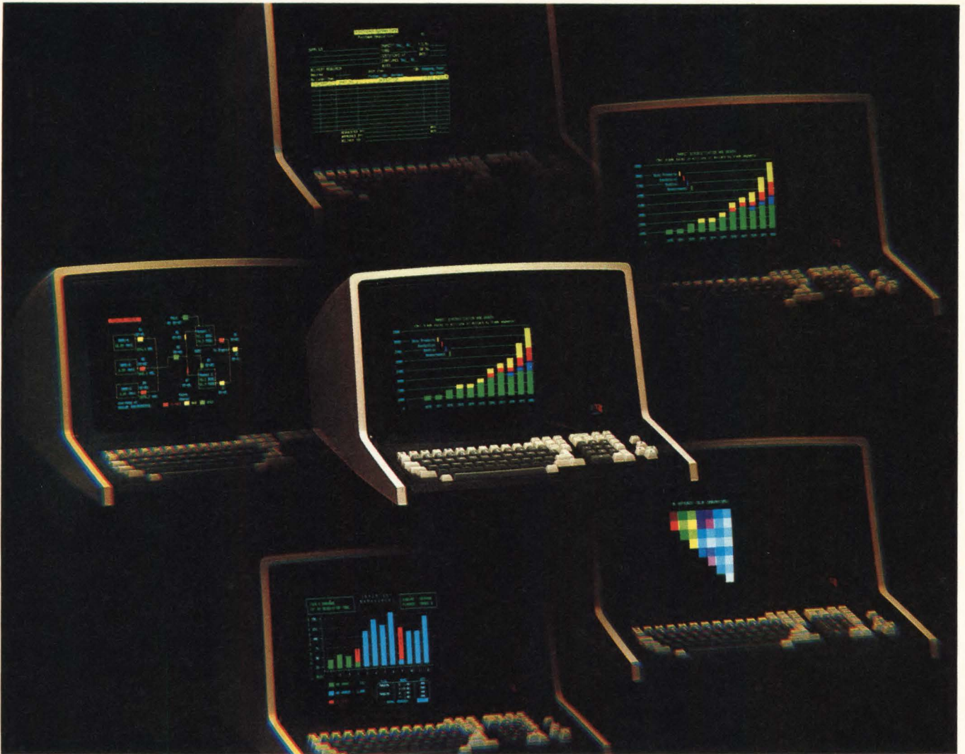
Figure 2: Intelligent Systems' Intecolor 2405 color terminal has ANSI X3.64, 80 \times 24 screen format with added color vectorgraphics and almost all the capabilities of DEC's VT100. Photo courtesy Ted Rodgers Studio; The Marcus Group, Atlanta, GA.
