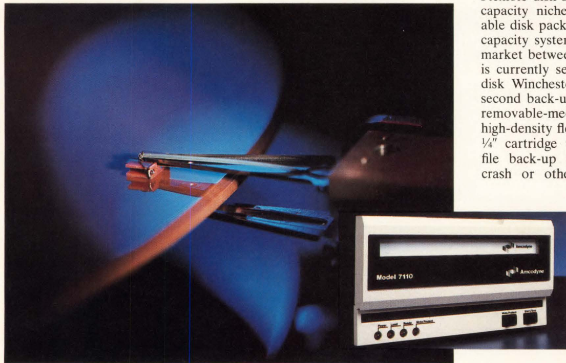
Figure 2: The Arapahoe 7110's low-mass mini-composite ferrite R/W heads are ramp-loaded onto the moving disk to decrease disk burnishing and increase data integrity.
