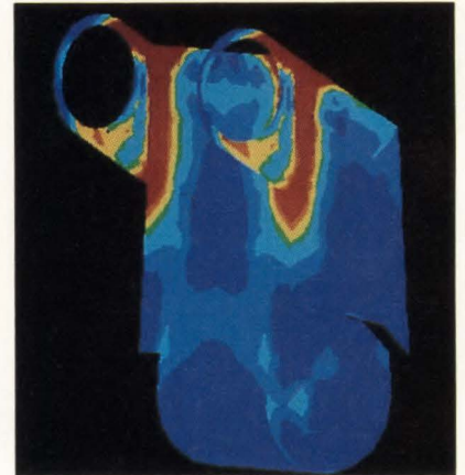
Figure 8: In a combination of design and engineering processes, color is applied to a model to provide the designer with information about stress. Photos courtesy GE/CAE International.
