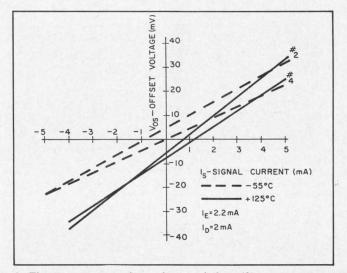
9. The temperature dependence of the offset voltage and dynamic ON resistance is not excessive for most applications. Two temperature extremes are considered, -55 °C and +125 °C.
