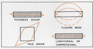
4. **Crystals may vibrate in four modes:** flexure, longitudinal (or extensional), face shear and thickness shear. In some cases, coupling is possible among the modes.
