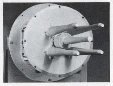
2. Dual-frequency Teflon feed receives at 4.12 GHz with the center element and transmits at 6.2 GHz with the four symmetrical elements.
