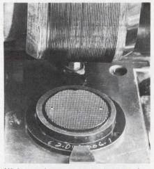
High-speed rotary saw dices wafers into over 1000 chips in 90 seconds.
