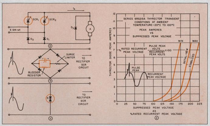
8. In a typical speed-control system (a), some provision must be made for protecting the SCR against voltage peaks and transients. Capacitor surge suppressors (b) and thyrector selenium suppressors (c) are commonly used.
