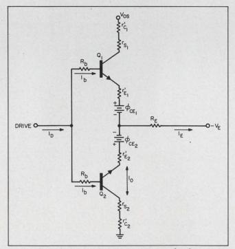
3. The equivalent circuit of a common-mode chopper includes the transistor offset voltages ( $\phi_{\rm CE1}$  and  $\phi_{\rm CE2}$ ). Being in opposition, these voltages tend to cancel, resulting in a low total offset voltage.
