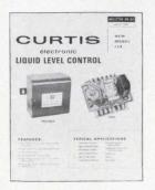
The Curtis LLS is a versatile, electronic static device incorporating a silicon-controlled rectifier (SCR) for operating the control relay. Operation is accomplished by sensing a minute current flowing between submerged probes. This AC current triggers the SCR and energizes the control relay. One set of control relay contacts allows internal pump-up or pump-down control, leaving two sets of contacts for the control operation function. Fully described and priced on new 2-page brochure DS-162.
