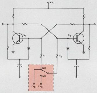
**Resetting of flip-flop** is easily achieved by an spdt switch connected to two power sources. This function does not require switching diodes.
