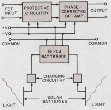
**Charging circuitry** prevents the batteries from overcharging and maintains charging currents under low ambient light levels.  $\pm 7.5$  V max at 10 mA. Unity gain frequency is 300 kHz min and the amplifier has 6 dB/octave slope from knee to unity gain. Open loop gain is typically 50,000 (30,000 min). Input noise is 4  $\mu$ V p-p.
