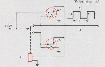
Low-frequency astable circuit is formed by three relays.  $K_{\rm 2}$  determine the ON cycle and  $K_{\rm 3}$  establishes the OFF period. Duration T is variable between four seconds and six minutes.
