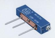
Type N hot molded adjustable fixed resistor rated  $\frac{1}{2}$  watt at 50°C ambient. Available with nominal resistance values from 100 ohms to 2.5 megohms with tolerances of  $\pm$ 10% and  $\pm$ 20%.
