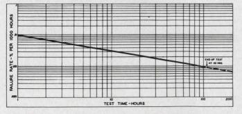
KEMET KG solid tantalum capacitors with predicted reliability are available from 0.0047 to 330 microfarads, 6 to 100 VDC, for continuous operation from -55 to 125 °C. Standard tolerances 10 and 5%. Closer tolerances on request.
