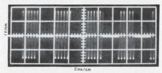
15. One-kiloHertz signal is chopped at 100-Hz rate. Center line is at zero volts dc.
