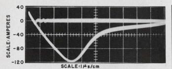
11. With high-duty cycles, diode recovery problems can interrupt the speed control, particularly when power transistors are used. Fast-recovery rectifiers should be used instead of conventional types. Note that the transient duration with the former (top trace) is only a small fraction of the latter (lower trace) and that the attendant current levels are much lower.
