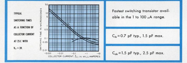
Sprague Electric also makes more than 200 standard SEPT<sup>®</sup> (Silicon Epitaxial Planar Transistor) Types, including 2N2218A-2N2222A, 2N2904A-2N2907A, 2N2369A-2N3209.
