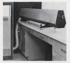
3. Commercially available  $CO_2$  laser system displayed by Korad Corp. reportedly provides a 75-watt output at 10% efficiency.
