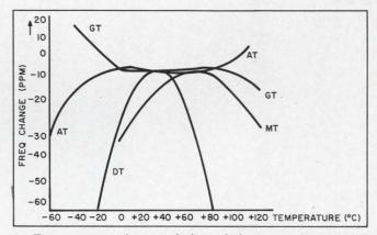
6. Temperature characteristics of four popular crystal cuts show the extremely stable behavior of the GT cut. Its frequency change is about 1 part per million over a  $100^{\circ}$ C range.
