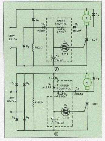
6. With shunt motors, speed control is effected by using the motor voltage to drive the SCR's phase-shift network. Shown are half-wave (a) and full-wave (b) control.
