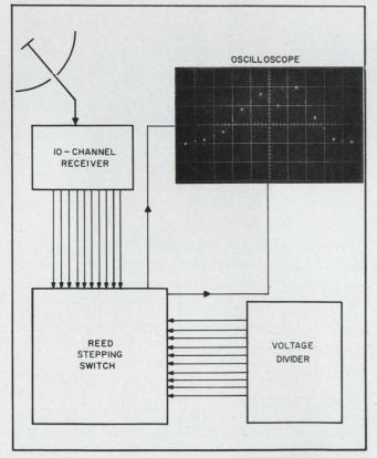
2. **Typical application** of the stepping-relay circuit is demonstrated by this arrangement for sampling the output of a multi-channel receiver.
