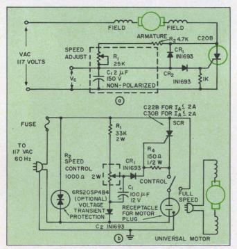
4. When an SCR is used to control the speed of a dc series or universal motor, it performs two functions: rectification and phase control (a). The  $R_1 C_1$  network establishes the triggering point of the SCR. To compensate for torque drops with decreasing input voltage, a more complex feedback arrangement is used (b). Here the voltage on the arm of potentiometer  $R_2$  is compared with the counter emf of the motor.
