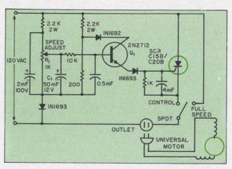
5. For wide-range, very smooth speed control a transistor is placed in the feedback path between the SCR gate and the reference adjust. Higher gain and stability result.
