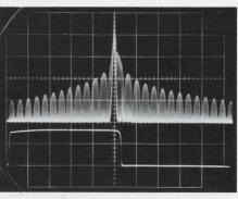
Time and Frequency Displays. The upper beam shows the spectral output of a 200 MHz gated oscillator applied as IF feedthrough to a Type 1L20 Spectrum Analyzer; the calibrated dispersion is 1 MHz/cm. The lower beam shows a real time display of the 10 kHz gating pulse; sweep rate is  $0.5 \ \mu s/cm$ .
