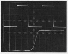
Sampling and Real-Time Displays. Upper beam shows a square wave at 1  $\mu$ s/cm as applied to a Type 1A2 Plug-In. The lower beam shows the risetime of the same pulse at 1 ns/cm as provided by a Type 1S1 Sampling Plug-in.
