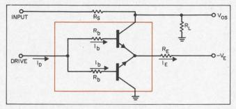
2. **Common-mode chopper** requires a good device match and a constant-current-source bias scheme. The outlined monolithic block provides an excellent device match.
