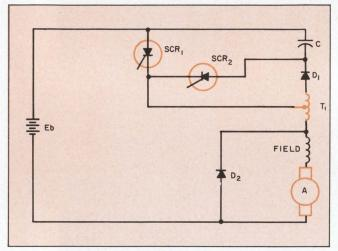
10. Reduction of the capacitor used in the chopper circuit is achieved by using an autotransformer. Here the capacitor is charged to higher voltages (than in Fig. 9b), to handle the same amount of joules  $(1/2 \text{ CV}^2)$ .
