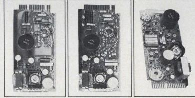
These printed-circuit cards (the magnetic operational amplifier . . . the magnetic square-root extractor . . . the magnetic multiplier/divider) are flexibly packaged in three standard types of case assemblies. In addition, completely programmed and packaged analog computer assemblies can be furnished to meet your custom requirements.
