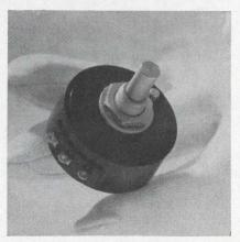
Models VS1/2 are miniature sensing switches featuring low hysteresis. The units combine silicon transistors and 1% metal film resistors in a welded cordwood assembly. With an input impedance of 8  $M\Omega$ , a 0.1- $\mu$ A input is required to switch up to 150 mA of output current. The switching level is factory set within  $\pm 1\%$ .
