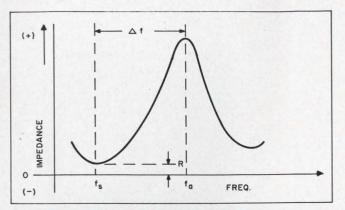
3. The impedance of a crystal is near zero at the series resonant frequency,  $f_s$ , and reaches its peak at the antiresonant frequency,  $f_a$ . Steep slope between these two frequencies indicates a high Q.
