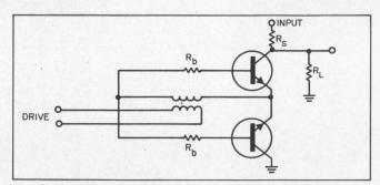
1. Conventional chopper circuit uses a transformer to isolate the drive circuitry from the signal channel.
