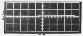
12. Chopper offset voltage is measured with zero signal voltage. The driver prf is 100 Hz and  $R_{\rm s}$  is equal to 10 k $\Omega.$ The center line is at zero volts.
