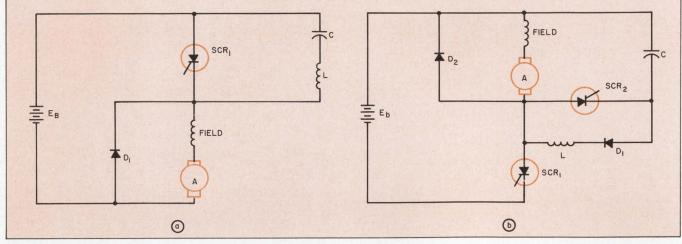
9. With dc power sources, SCR chopping is used to frequency-modulate the power supplied to the armature (a). When an extra SCR is used for pulse-width modulation (b)
