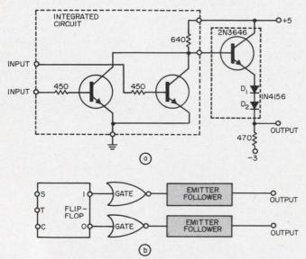
Noise immunity is increased when an emitter-follower diode output stage is connected to an integrated circuit (a). Suitable for DTL, TTL and other logic elements, they are used with buffer-gates when connected to flip-flops (b).
