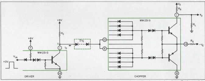
10. **Complete driver-chopper circuit** uses two WM231G devices. The series-string of diodes is used to provide a
