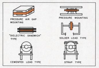
5. The mounting technique for crystals depends on the particular application. The most widely used methods are shown above.
