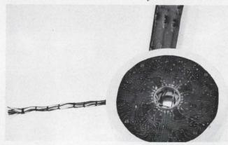
Shrinkable tubing encapsulates modules of various sizes, providing insulation and environmental protection, and even binding the modules together.
