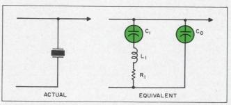
2. Equivalent circuit of a crystal includes the capacitances contributed by the wire leads and the holder in  $C_o$ . The ratio of  $C_o$  and  $C_1$  indicates the frequency separation between the resonant and anti-resonant frequencies of the crystal.
