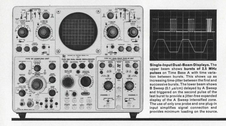
Here's a new Tektronix Oscilloscope that will tackle virtually every measurement job in your laboratory. The Type 556 and its rack-mount counterpart, the Type R556, have an ability for simultaneous information display that makes complex measurements simple and routine. They accept any Tektronix letter and 1-series plug-ins, including spectrum analyzer and sampling units.
