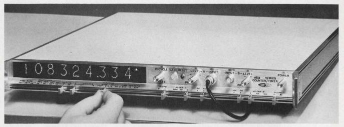
Frequency counter stacks up 1-3/4 inches tall. Using front-panel slide-switch controls
