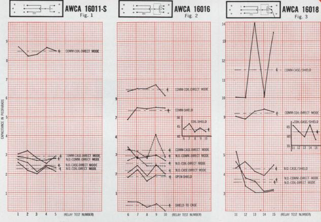
Data was obtained using a Boonton Electronics Corporation Capacitance Bridge, Model 75-A-S8 at 1MH2
