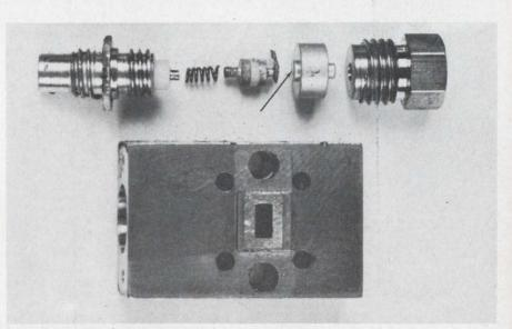
LSA waveguide circuit—less wave-guide short and E-H tuner—is shown with inner components. Arrow shows GaAs mounted on heat sink.
