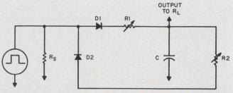
Switching D1 and D2 with the input pulse permits independent rise-and-fall-time control.
