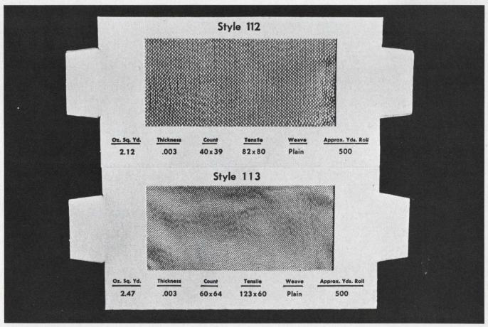
2. Tighter weave fiberglass (style 113) will resist movement while looser weave (style 112) may tend to move
