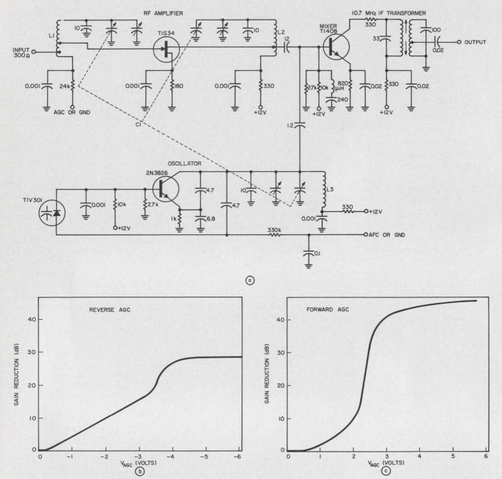
3. Replacing mixer FET with a bipolar results in worse tuner performance. Both reverse (b) and forward (c) agcs
