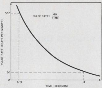
3. Pulse rate is plotted as a function of time. Digital techniques can be used to produce an accurate record of this curve. Actual data obtained are shown in the Table.
