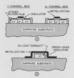
Isolation b e t w e e n complementary transistors is achieved by selective removal of silicon (a). The same technique is used to leave interconnection conduits for crossovers.
