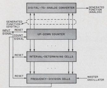
2. Time functions can be generated digitally with a system such as this. Flip-flops are used for both interval-determining and frequency-division cells.
