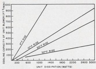
2. Temperature inside a black box increases about  $10^{\circ}$ C ( $18^{\circ}$ F) for every 5 watts dissipated when the blower delivers 1 ft³/min of air over the equipment. These curves are based on this approximate relationship.
