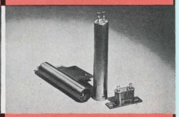
Cartridge Type: Series C8 hermetically sealed and still adjustable. Contact rating up to 5 amps. Crystal Can Size: Series VE-2 hermetically sealed. Contact rating up to 3 amps. Features: Rapid rate of response; minimal differential; operating range, —65° to +300°F; vibration to 2000 Hz; shock to 50g.
