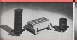
G-V is the largest source and offers the widest variety. Several types are hermetically sealed and still adjustable. All meet requirements of Mil-R-19648. Available in a wide variety including: subminiature, miniature, octal and missile types. Features: delay time, 0.1 sec. to 3 min.; heater voltages to 230 V; ambient operating temp., —55°C to +125°C; vibration to 2000 Hz; shock to 50g.
