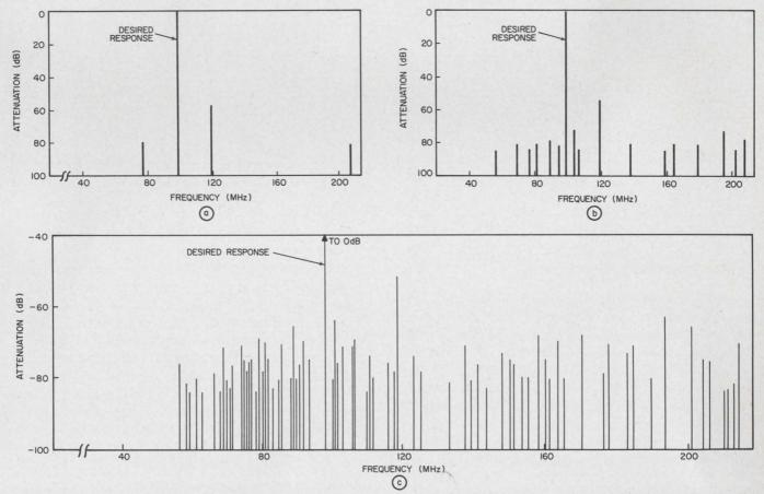
2. Only three spurious responses below 85 dB were observed with the FET-RF and FET-mixer tuner (a). This
