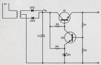
1. A collector-to-emitter short in Q1 will cause  $\rm V_{in}$  to appear at the supply output terminals, destroying an entire IC system.
