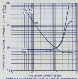
NORMALIZED COMMON BASE CHARACTERISTIC VS. COLLECTOR CURRENT
