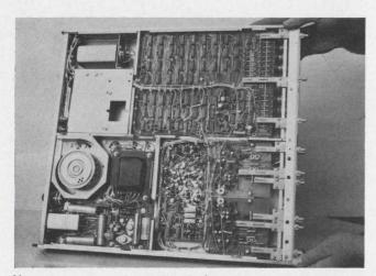
How to cut panel height. Horizontally mounted board (upper right) holds all ICs. Even the squirrel-cage blower and the transformer (lower left) fit the 1-3/4-inch-high package. Tabs extending in from right are switch leaves for the slide switches.
