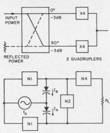
Unilateral quadrupler circuit (above) contains a center-fed balanced-pair quadrupler in each arm. Each is fed from a 90°, 3-dB hybrid.
