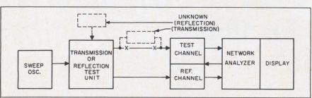
1. Block diagram of the complete network analyzer system adapted for either transmission or reflection measurement of microwave devices.
