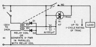
3. High transient currents are switched without bounce by the Triac while the relay contacts take on the continuous operation. Voltage drop across the contacts is only about 1 volt during both closure and opening. For inductive loads RC arc suppression in parallel with Triac should be employed.
