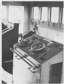
**Bridge** console in General Electric system allows complete control of the ship's propeller speed from "full ahead" to "full astern."
