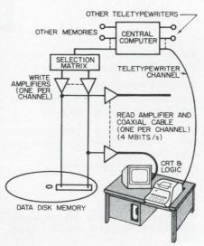
Remote display consoles for timeshared systems, like the one shown schematically here, could be built for less than \$10,000 each, according to the Bell Telephone Laboratories engineers who designed it. NEWS
