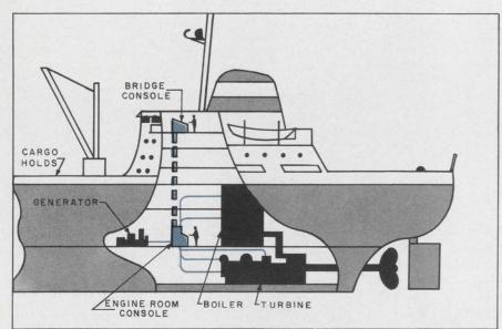
Centralized control of ship's power plant is maintained from two points: the bridge and engine-room consoles. Dotted line is the main interconnection between consoles. Solid lines indicate loops to sensors and actuators.
