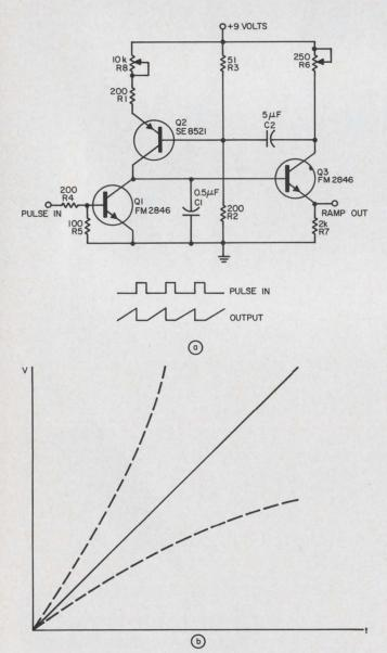
Potentiometer R6 in the output stage of the ramp generator (a) is used to vary ramp linearity as demonstrated in (b).
