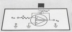
TC -200 ppm/°C. They are available in any value from 0.001 to  $0.100\mu\text{F}$ , 50 VDC, with tolerances as tight as  $\pm$  1%.
