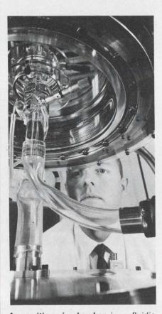
A sensitive air chamber in a fluidic gyro responds to motion changes by forming detectable vortical patterns.
