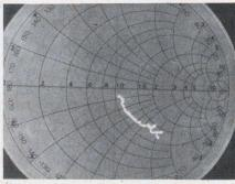
2. Smith chart overlay with trace shows impedance characteristics of microwave pellet transistor with common-emitter configuration.
