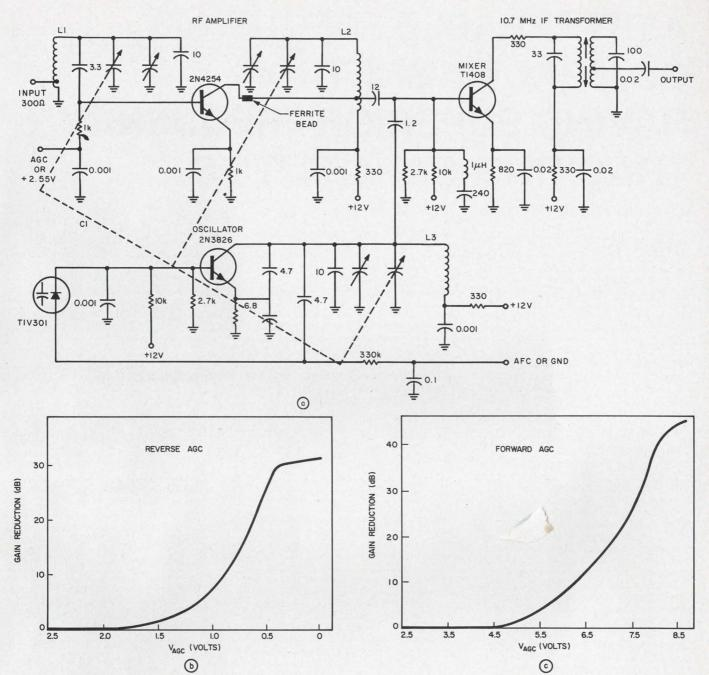
4. The over-all tuner performance is degraded even more when all FETs are replaced by bipolars. Note that the ago
