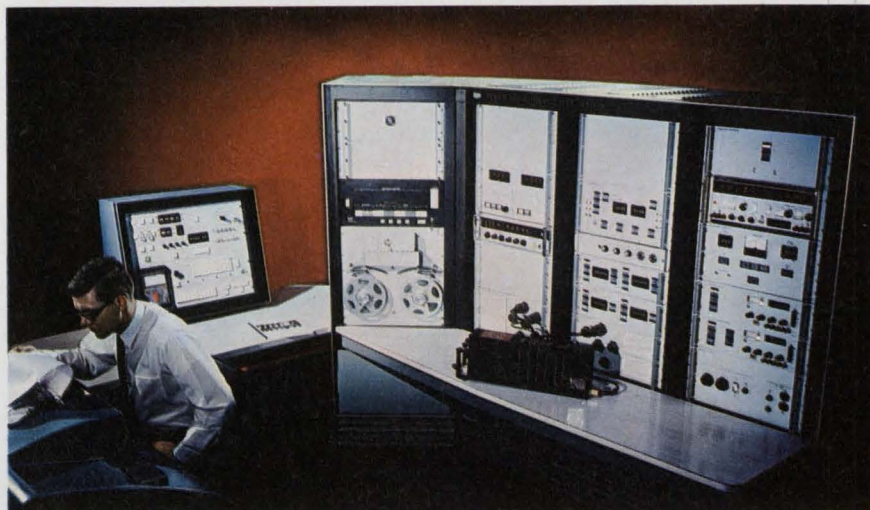
Airlines are increasingly going to computer-controlled test systems to check out their complex avionics equipment. Bendix Corp.'s test system shown above is the subject of Wescon paper 21/3.
