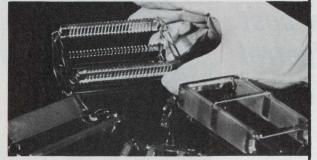
Newly designed carrier boats from Amersil are a marked improvement over slotted plate and slotted rod carriers for low and high temperature diffusion applications. This construction provides more secure wafer spacing for uniform diffusion.
