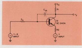
white level. The gain may be adjusted by changing either the collector resistance,  $R_1$ , or the emitter resistance,  $R_2$ , with a potentiometer. These potentiometers have an appreciable amount of stray capacitance that, in the collector circuitry, adds to the load capacitance. For this reason it is often preferable to place them in the emitter circuitry. There, the impedance is so low that the additional capacitance has no significant effect.
