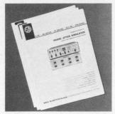
Simulation of the existing telephone channels has become exceedingly important as data transmission increases. For testing, training and evaluation, controlled impairments must be introduced. These include Phase Jitter, attenuation and envelope delay distortion, impulse hits, broadband noise, harmonic distortion and phase hits. SEG's new bulletin on the Phase Jitter Simulator
