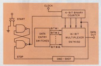
2. A multiplexer is used as the basic storage element in this 16-bit word generator. The outputs of the data entry switches are always available at the inputs to the multiplexer. Once the start button is depressed, the counter controls the sequencing of the multiplexer.
