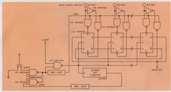
1. The simplest form of programmable word generator uses flip-flops to form a presettable shift register. This word generator is easy to build and is extremely useful
