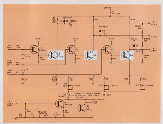
8. This complete RGB video amplifier uses a single shunt inductor for frequency compensation. Note how the low-impedance luminance preamplifier,  $Q_1$  and  $Q_2$ , of Fig. 7 is used to prevent chroma cross-coupling. The low-pass R-C filters on the three color-difference inputs are needed to attenuate the 3.58-MHz chroma carrier. And
