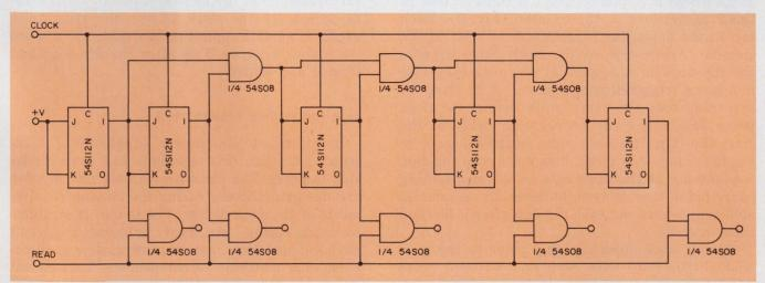
2. The features of both the synchronous and ripple counters are combined in a counter whose speed is limit-
