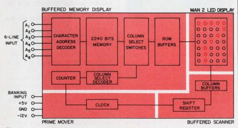
The MDA111 LED display package has four sections: a buffered memory display with a six-line input, a clock with a blanking input and power supply voltage lines and a MAN-2 35-dot LED display.
