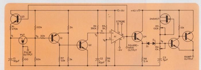
This multifunction low-frequency generator supplies three signals at the same time. The dc level of the
