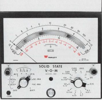
1. Lower power ohms — 8 ranges with 35 mV power source and 1 ohm center scale.
