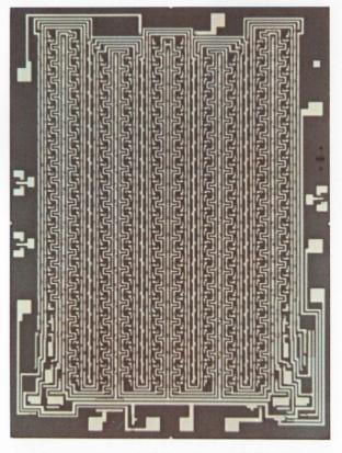
Dual 100-bit static shift register — MC1160G
