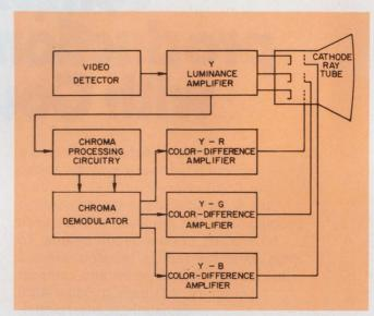
1. The color-difference circuit needs a powerful luminance amplifier that requires not only a high-power transistor but a large heat sink as well. It has the advantage of providing identical luminance transient responses for all three colors, thus eliminating a source of color fringing.
