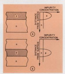
1. Layers of impurity concentrations can be implanted at the surface of a substrate (a) or buried inside (b).
