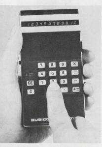
Battery operated pocket calculator will have a light-emitting diode display.
