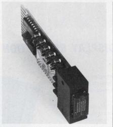
A complete alphanumeric LED display consisting of a 35-dot matrix readout and all the necessary driving circuitry in one package can now be purchased at \$68 in OEM quantities.
