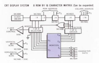
to terminal equipment requirements are new developments in products for terminal receivers and transmitters and for CRT display systems.
