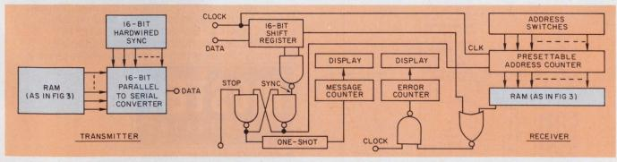
4. Two simple programmable word generators form a bit-error detector. The transmitter produces the test signal that is applied to the system under test. The sys-
