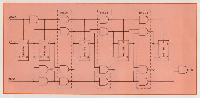
3. A simple modification of the synchronous/ripple counter of Fig. 2 can increase its speed beyond that of the synchronous counter. By applying both the clock and
