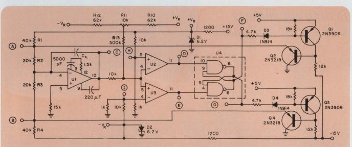
1. This versatile function generator provides triangular, square-wave and pulse outputs for less than \$50. The circuit employs only four ICs, four transistors and a few other components. Its triangular output can be finely controlled with respect to frequency and slope.
