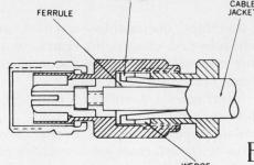
This Emlock cable grip of ours is all metal and offers the advantages of compression back ends with assembly time equal to crimp. As a clincher, it's impossible to pull the cable out of an Emlock connector. Disengagement will be caused
