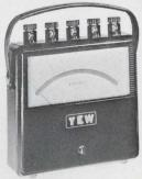
There are many other words that describe our complete line of portable standard instruments, too — like rugged, versatile and available. Yokogawa Electric has over 55 years of experience in the manufacture of precision instruments and is now introducing this complete line of taut-band portable standards
