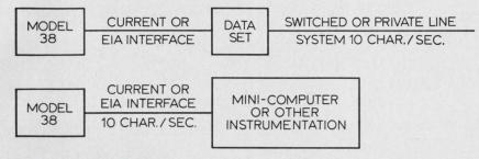
A second interface option is really two options in one. The set is equipped with both a voltage interface that conforms with EIA Standard RS-232-C and a current interface of 20 or 60 ma.
