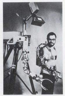
Slave arm imitates motions made by master arm on the operator by equalizing potentiometer readings on both.
