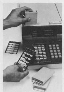
function blocks include separate (ROM) memories so they do not draw on the main calculator memory, leaving it fully available for further problem-solving power. A third keyboard plug-in option, the User Definable Function block, allows you to customize individual keys for operations uniquely important to you and your discipline.
