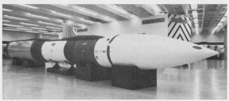
Boeing-built mockup of the Air Force Minuteman III, newest version of the three-stage solid fueled ICBM, shows its bullet shaped shroud, which covers its re-entry system.
