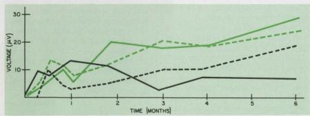
A new low-cost FET op amp features low voltage drift even over long periods of time. Four such model ZA903M2 op amps were tested over a six-month period for drift-vs-time characteristics. The average voltage drift was  $\pm 10~\mu V$ . Corrections were made for temperature variations.
