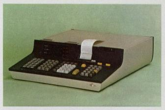
Hewlett-Packard's Model 10 calculator packs a lot of computing power in a fairly small package. The modules included with the calculator allow the user to set a group of special function keys to perform a variety of calculations at the push of a button.
