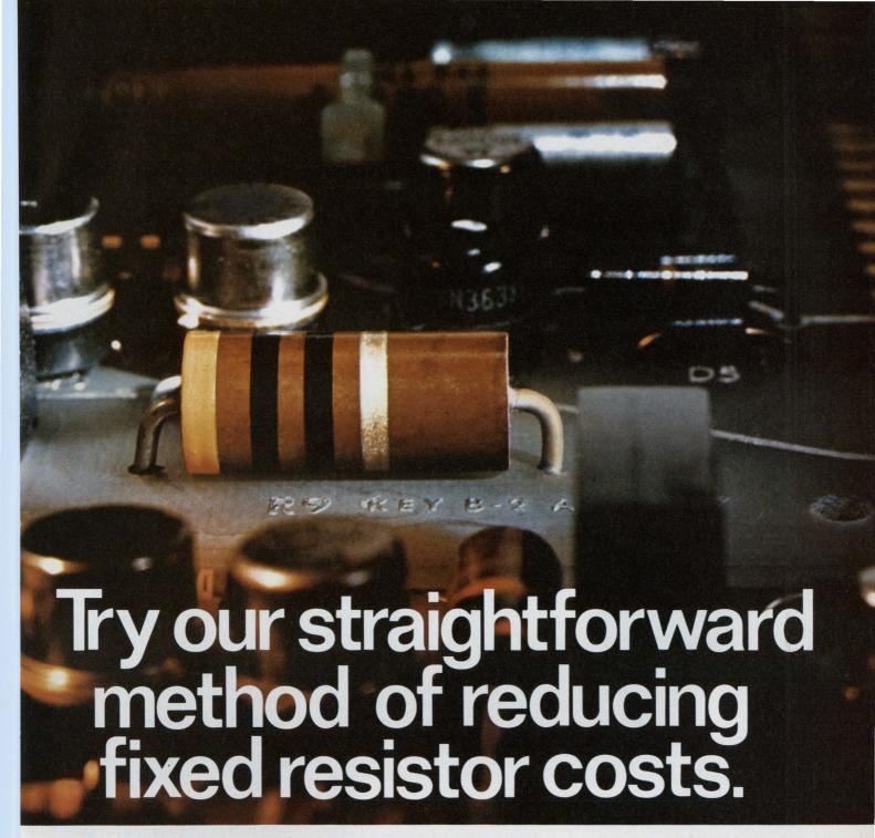
You can't blame engineers or purchasing agents for trying to save every last penny on resistors these days. But lowest price doesn't necessarily mean lowest cost. For example, most manufacturer's color bands won't stand up to the cleaning methods used to remove excess flux. Or they darken and become illegible from the heat
