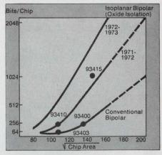
The graph gives you some idea of where we've been and where we're going with bipolar memories and isoplanar. It indicates the feasibility of 2048 and 4096-bit read/write memories for 1973. By then we fully expect isoplanar to dominate memories in high-performance and small systems. Memory designers please note that our estimates of packing density and time scale are at least as conservative as our original announcement of the process.
