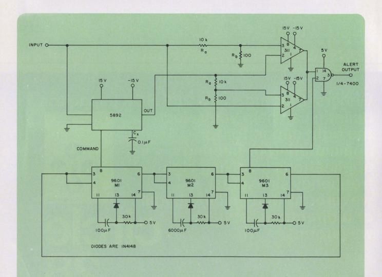
An output of logic ONE indicates a changing input. But when a logic ZERO appears at the output, the
