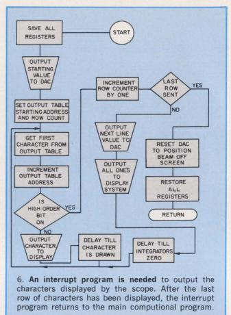
from computer to computer. In general, an interrupt program (Fig. 6) is needed to output a table of characters periodically for display, and a table lookup program or subroutine is needed to decode internally generated information to the display character codes. Of course, a main program is also needed to specify what data is to be displayed and to format the data into characters per line and lines of characters.
