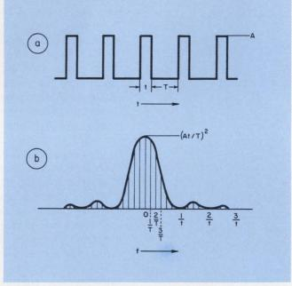
1. The sampling function can be described in two ways: In the time domain, it is a periodic gate function (a), while in the frequency domain, it is a series of spectral lines under a  $[(\sin x)/x]^2$  envelope (b).
