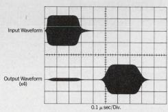
Typical waveforms for a 0.5 microsecond delay line driven by a 0.25 microsecond pulsed carrier at 60 MHz.
