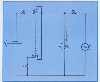
1. Switching can reduce back intermodulation, provided that resistances  $r_1$  and  $r_2$  are equal. In this model,  $V_i$  and  $R_i$  represent an interference source.
