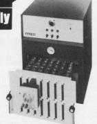
The INRECO static handling system is a must for testing I.C.'s, diodes, transistors, resistors, etc. Devices are clipped to special test P.C. cards which are inserted into inner door mounted connectors. With the door in place and the required temperature in the chamber, all the devices may be powered and/or sensed individually by the scanner plugged into connectors on the door exterior.
