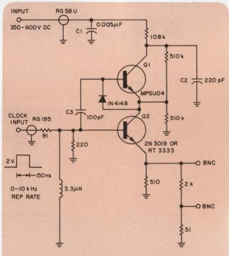
Two transistors in an avalanche mode are used as the basis for this fast, high-current pulser. A clock input provides the means for synchronizing the output pulses. The output load is 50  $\Omega$ .
