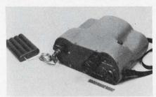
Laser rangefinder being tested by the Army. The small, rectangular display to the right of the eyepiece shows the range in meters in light-emitting-diode digits.
