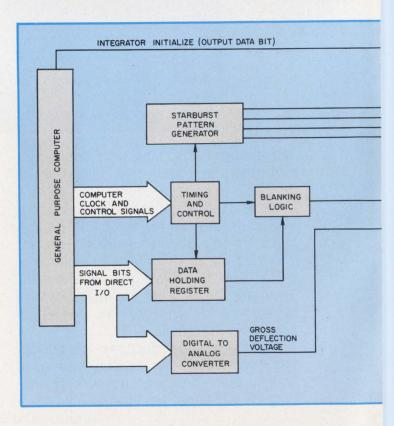
burst cycle (all others are reset). This ONE is shifted down the register at clock rate, generating the 22 stroke times. (The register can be connected as a ring counter and the display run continuously, but synchronization with the external commands becomes more difficult.)
