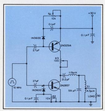
2. This experimental switched amplifier has enough bandwidth to pass both the interference and intermodulation frequencies. To reduce the amount of back intermodulation, resistor  $R_{\rm 3}$  is adjusted to equalize the ON resistances of the two transistors.
