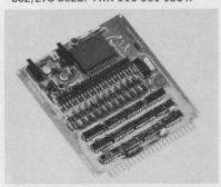
ADC 300 Series Converters. Complete, fully-assembled, plug-in modules incorporate all of the functions necessary to perform conversions except for power supplies. Accurate to within  $\pm 0.025\%$ . Single card open construction facilitates field repair and low profile permits units to mount on 0.5" centers. Price of the ADC 312 (12 bit) unit in 1 to 5 quantities is \$300. Phoenix Data, Inc., 3384 W. Osborn Rd., Phoenix, AZ 85017. Phone 602/278.8528. TWX 910-951-1364.
