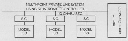
You can even use the model 38 in multi-point "selective calling" systems by adding a Teletype Stuntronic $^{\text{TM}}$  station controller.
