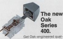
ity in keyboard switches with the inherent reliability of electromechanical operation. Ideal for peripheral data-processing equipment. Contact bounce is less than 3 milliseconds. Long life, up to 20 million operations per key. Designed with self-cleaning crossbar-wiping contacts.
