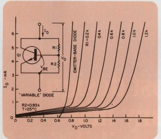
"Variable diode" schematic provides clamping voltages between those that are obtained from one and two common diodes. The curves relate  $I_{\rm D}$  to  $V_{\rm D}$ .
