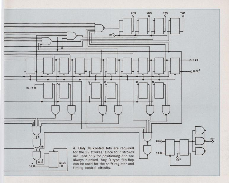
once the clock frequency of the starburst pattern generator is established and the maximum number of characters per line is decided upon, the integrating capacitor should be chosen so that only the required number of characters per line can be written before the integrators saturate. In this way the minimum value for the capacitors will be chosen. With a minimum capacitance, the integrator reset time is kept to a minimum.
