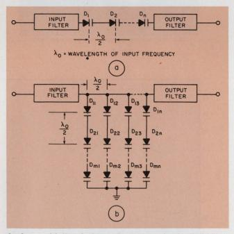
2. Any multiplier design reduces to a simple diode-filter combination (a). For the 80-W multiplier, the equivalent circuit is represented with discrete components (b). Capacitors  $C_4$  and  $C_6$  and inductor  $L_5$  provide diode-input matching. At the output is a cavity filter.
