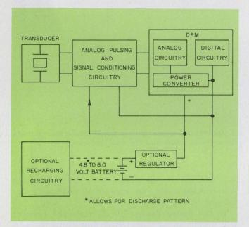
5. A portable, battery-operated instrument, such as this ultrasonic thickness gauge, is a natural application for a five-volt-powered DPM.
