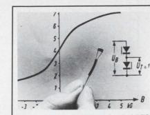
EEP AHY10 MAGNETIC DIODES change internal resistance as function of external magnetic field. AHY10A passes 1mA at BV with sensitivity of 0.75 — 1.0V/kG. Four types. Numerous uses. 8-page application note, full data avail-able: European Electronic Products, 10180 W. Jefferson, Culver City, Ca. 90230 213/838-1912
