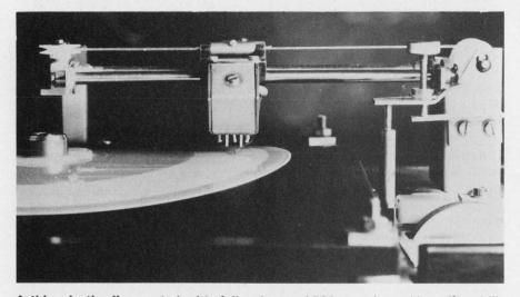
A thin plastic disc coated with foil spins at 1500 rpm in making video hilland-dale recordings in Teledec's system. Single-disc players and automatic changers with two hours playing time are under development.
