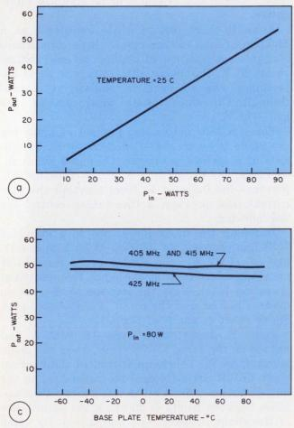
4. Measured results of the multiplier design reveal a linear input/output power variation (a) and a 1-dB bandwidth of 14% (b). Operation up to a base-plate temperature of 80 C is possible (c), while VSWR over the -60 to 90 C range is held below 1.22:1.
