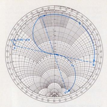
3. The calculation of the input matching elements, C<sub>4</sub> and L<sub>5</sub>, is performed graphically with a Smith chart. All that's needed to start the calculation is  $Z_A$ , one-half of the input impedance of a diode.
