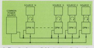
6. **Five-volt units are called for** in this application, where multiple displays are fed by independent signal sources. Considerable saving results from the use of a common power supply.
