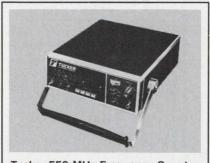
Tucker 550 MHz Frequency Counter. 9 full digits with a resolution of IHz the Tucker 5509 Counter is a tiny, low-cost and simple to operate Counter. Aging Rate is  $1 \times 10^{-5}$ /day. Price \$950. Send for free catalog. Tucker Electronics Company, P. O. Box 1050, Garland, Texas. (214) 348-8800.
