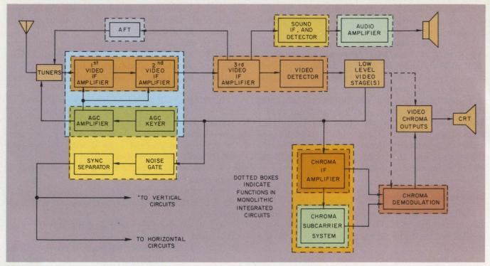
**ICs are being used in color television receivers** to perform several subsystem functions. The ICs, indicated by dotted boxes, can provide complex circuits and better
