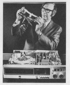
The precision tape transport is a vital component of RCA's new Mag-Tape cartridge video recorder.
