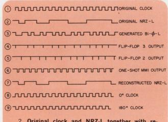
2. Original clock and NRZ-L together with reconstructed waveforms, illustrate the components of biphase-level PCM.
