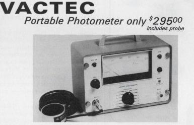
High sensitivity, wide range .001 to 10,000 fc. ● Accuracy 5% full scale, linearity 3%. ● AC or battery operation. ● Recorder output (1 v. to 1 ma. output).
