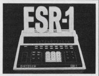
Dietzgen's new 12-digit electronic slide rule does even more than your slide rule. All trig. and exponential functions—including hyperbolics and natural log—with a single function key. Converts degrees, minutes, seconds to deċimal; degrees to radians or vice versa. Dietzgen Corp., 2425 N. Sheffield, Chicago, 60614. (312) 549-3300.
