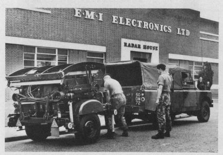
Highly mobile mortar locating radar developed for the British Army is mounted on a two-wheeled trailer.
