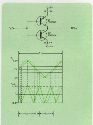
**Each input signal peak** produces three output signal peaks with this nonselective tripler circuit. The additional peaks occur where the input signal causes saturation of one of the two transistors.
