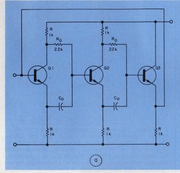
3. A "series-resonant" circuit is built with two phaseshifting networks (a). Capacitor values depend on the desired resonant frequency. Transistors should have high
