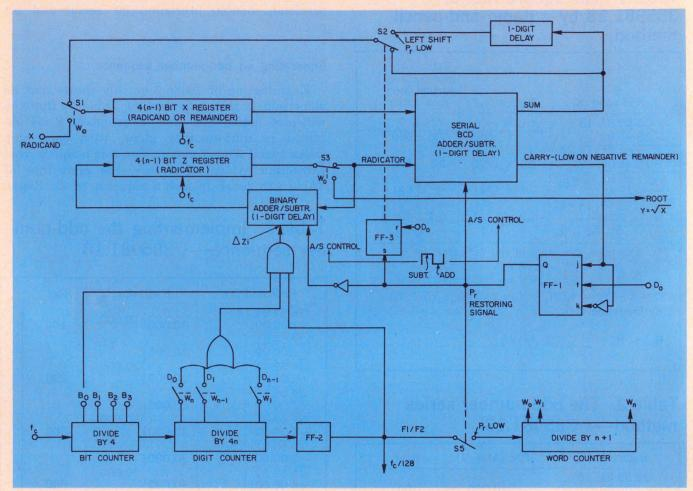
1. A square-root extraction circuit has many features in common with a divider system. The odd-numbersequence radicator that is generated in the Z register
