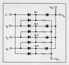
In this circuit we have  $M_1 = Max (V_1, V_2,), M_2 = Max (V_2V_3), M_3 = Max(V_3, V_4)$  and  $M_4 = Max (V_4, V_1)$ , as well as  $V_0 = M_{1n} (M_1, M_2, M_3, M_4)$ . If  $V_1 < V_2 < V_3 < V_4$ , as assumed in the article, then  $V_0 = V_2$ , the second-smallest value as desired. However, if the levels for  $V_1$  to  $V_4$  are 1, 3, 2 and 4, then  $M_1$  to  $M_4$  are, respectively, 3, 3, 4 and 4, and  $V_0$  equals three, which is incorrect.
