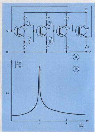
4. "Parallel resonance" is obtained by the addition of another phase-shifting network with a fixed  $180^{\circ}$  phase shift (Q<sub>3</sub>). Component values depend on the transistors selected and on the desired frequency. Approximately the same values as those for Fig. 3a can be used. Note, however, that this circuit exhibits a considerably higher impedance-ratio peak than that of Fig. 3a.
