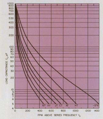
3. The degree to which a crystal can be varied in frequency depends upon the ratio of the motional capacitance  $C_1$  and stray capacitance  $C_0$  as well as the Q of the device. Variations of bandwidth are shown.
