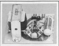
5 watt regulated power supplies. Low cost power supplies designed around 7800 series of voltage regulators, these units are available in 5, 6, 8, 12, 15, 18, and 24 volts with a 5 watt output rating. Short circuit protected. \$9.75 in unit quantity. ELCOM Industries, Inc., Civil Air Terminal, Bedford, Ma. (617) 274-6656.
