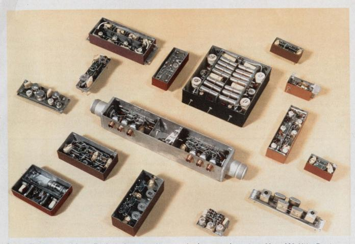
**Crystal filters** are used in applications where very sharp bandpass or band-reject characteristics are needed. Operating frequencies of these filters, by McCoy Elec-
