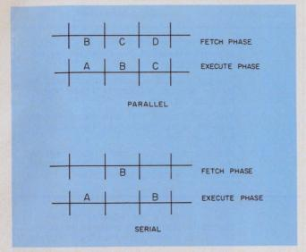
4. Micro-instruction sequences may be parallel or serial. In a parallel approach, one micro-instruction can be executed while the next one is fetched. However, in the slower serial sequence, completion of a micro-instruction is required before the next one can be accessed. Letters shown denote micro-instructions.
