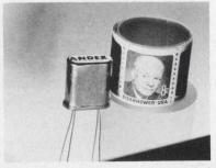
Ceramic bandpass filter and oscillator control resonator with excellent frequency stability. Used in remote control, low frequency navigation, underwater signalling. From 6 kHz to 200 kHz. Loss 5 dB, 0.9% min. 3 dB BDW, 20 dB/3 dB skirt ratio <13. ANDEX CORPORATION, Middleburg Hts., Ohio (216) 845-1953
