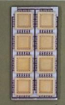
These eight AlSiPak<sup>®</sup> 24lead hermetic chip carriers on AlSiBase<sup>®</sup> multilayer ceramic substrate give far greater circuit density.
