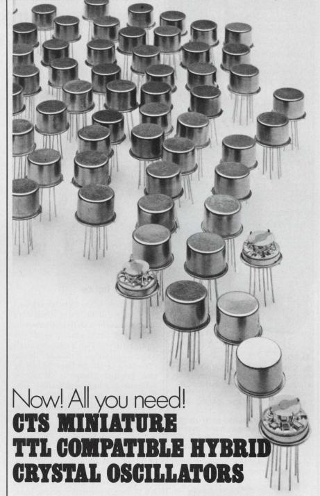
NEW CTS TO-8 crystal oscillators eliminate one of your biggest design headaches . . . size . . they're in a compact .07 cu. in. package. They feature a coldweld enclosure and reliable hybrid circuitry. Frequency range is 500 KHz to 25 MHz. Available as complimentary, multiple binary related outputs capable of driving 5TTL. Temperature stability:  $\pm$  25 ppm 0°C to 70°C.
