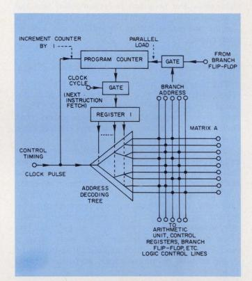
2. One matrix can be eliminated when a semiconductor ROM and program counter are used. The next address is obtained by the program counter, which is incremented by one after each new micro-instruction is fetched.
