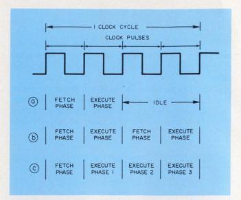
3. Monophase and polyphase timing have different fetch and execution sequences. Monophase cycling can be inefficient because of unused clock periods (a). The efficiency can be improved (b), but a polyphase approach provides the fastest processing time (c) at the expense of greater complexity.
