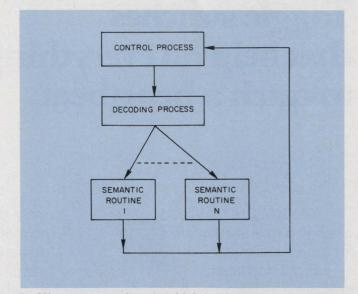
6. Microprogramming for high-level language processing. This approach, and efficient microprogramming, can avoid the need for costly compilation to a lower-level assembly language.
