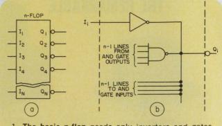
1. The basic n-flop needs only inverters and gates to produce stable outputs for pulse-inputs.
