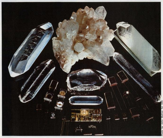
Quartz crystal wafers, sawed from synthetically grown quartz boules, are polished and mounted in a variety of packages, including glass. Electrodes are plated or de-
