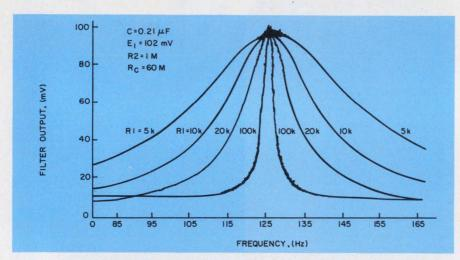
3. The bandwidth of the commutative filter is adjusted by simply changing the value of input resistor  $R_1$ . In practice, this may be a potentiometer.
