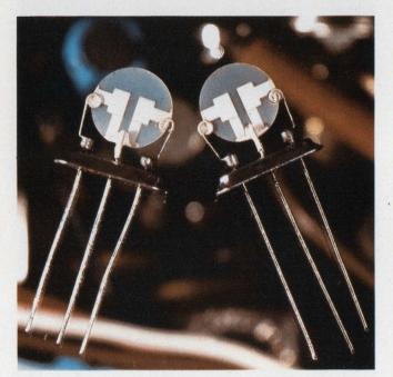
These two-pole, **21.4-MHz monolithic filters** by Piezo Technology are ultraminiature. Four, six and eight-pole filters are made using multiple two-pole units.
