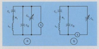
2. With ideal crystals and generators, these circuits produce the same frequency for a given value of  $C_{\rm L}$ .
