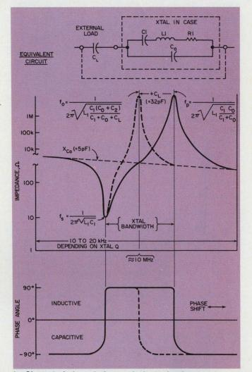
1. Characteristics of the equivalent circuit of a quartz crystal are such that when operating at series resonance  $f_{\rm s}$  the reactive components of  $C_{\rm 1}$  and  $L_{\rm 1}$  are equal and the load is resistive. At the antiresonant frequency  $f_{\rm p}$  the crystal presents a high inductive reactance.
