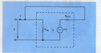
1. The basic transistor feedback circuit, with the amplification factor, F, dependent on frequency, serves as the model for building subsequent "series" and "parallel" resonance circuits.
