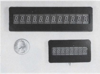
**Multidigit fluorescent readouts** from Ise Electronics lend themselves to easy multiplexing and provide a soft green glow.
