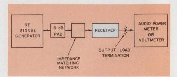
1. **Receiver quieting can be measured** from a simple setup. However the technique can't distinguish between i-f and audio response.
