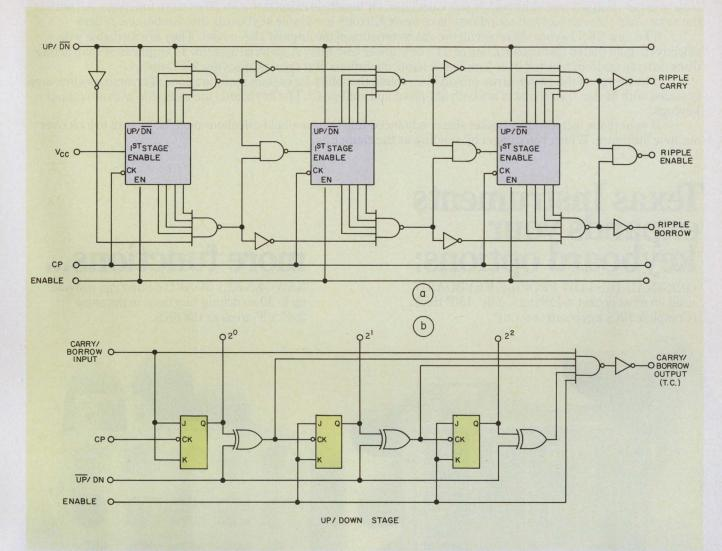
12. Circuits for the enabling of up/down counters are similar to those used with "up" counters. The main difference is that a second enable chain is used for the
