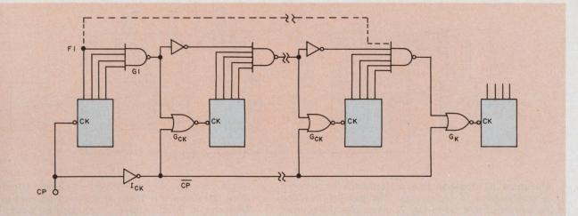
5. Greater clock speeds can be used if the clock-line is also enabled. Both the gate-inverter delay and the 1-to-0 transition delay of  $F_1$ —at each clock pin—are elimi-
