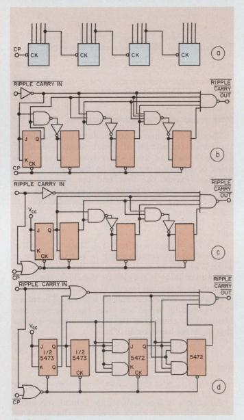
7. Synchronous sections boost speed. The ripple connection (a) is the simplest for multisection counters. Each stage (flip-flop) must be enabled at the same time since they are all toggled by the clock (b). Enabling the clock simplifies the circuitry (c) and (d). Similar circuits are available as MSI sections.
