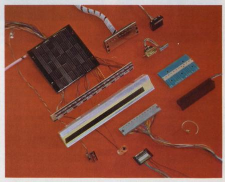
Simple and complex photosensing devices and arrays, by Sensor Technology, are used for optical decoders and for computer punched card and punched tape readers. Some devices have hybrid amplifiers for TTL interfacing.
