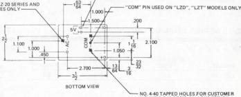
NO. 4-40 TAPPED HOLES FOR CUSTOMER MOUNTING (2 REQ'D ON LZ-10 SERIES) (3 REQ'D ON LZ-20 & LZ-30 SERIES)
