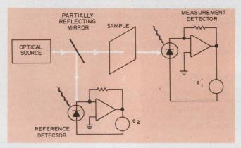
2. A reference detector, which delivers a signal proportional to the incident-intensity level, has been added to the straightforward system of Fig. 1. The new signal can generate a source-variation correction term.
