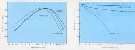
Single-crystal ferrite tape heads from Fuji Electrochemical provide much longer life than conventional polycrystalline ferrite or permalloy heads and extend record/playback response to higher frequencies at a small sacrifice in the lower frequencies.
