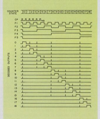
11. Glitches can occur in the identification (or decoding) of synchronous counter sections. Some of these spikes can occur on counts that precede the identified state, which is not the case with simple ripple-counters. Any of the enabling techniques gives rise to the possibility of such spikes.
