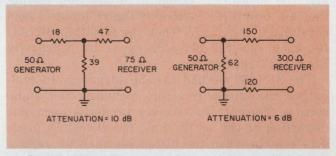
4. Simple impedance matching pads can be built to provide a wide range of attenuation values.
