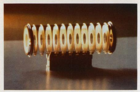
A new supersensitive solid-state photomultiplier, by Electronic Vision Corp. focuses electrons from a photocathode onto a silicon array. Each of the electrons striking the silicon is multiplied by several thousand.
