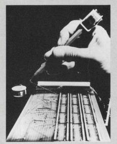
A special pen that issues wire from its tip speeds up circuit construction in Siemen's new breadboard system.
