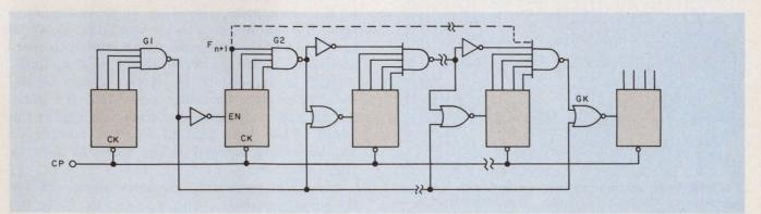
2. Apply parallel enabling from all flip-flops in a single section and you are using the terminal count—as generated by the multi-input AND gate. The same 74L30
