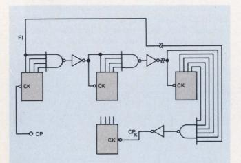
4. Clock-timing restrictions are removed with this configuration of MSI ripple-counters. The signal from  $F_1$  the first flip-flop stage of the first section—becomes the virtual or secondary clock for the counter. The addition of  $F_1$  to each counter section eliminates the 1-to-0 ripple delay of the gates.
