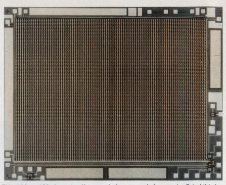
This 100  $\times$  100-element self-scanned charge-coupled array, by Fairchild, has an image aspect ratio of 4  $\times$  3. The charge coupling uses buried channels.
