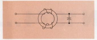
3. Common-mode interference can be reduced with a simple, "common-core" line-to-line filter.
