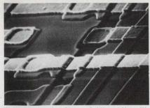
This is the surface of Hitachi's silicon-gate MOS chip for an 8-digit calculator with memory.
