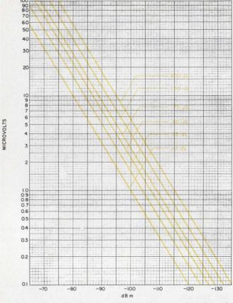
9. Conversion of dBm to  $\mu$ V for a given receiver impedance can be performed with this graph.
