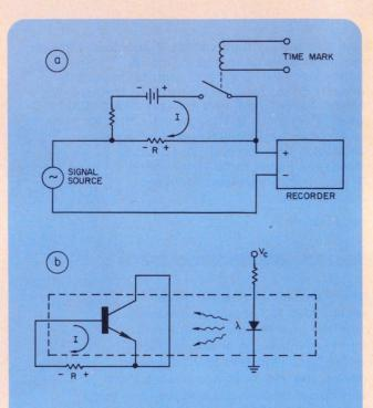
1. The battery-relay combination is often used to add a time-mark capability to chart recorders (a). The components in the dotted line can be replaced by the phototransistor connection (b), which generates the required offset voltage.
