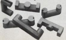
Tektronix, Inc. selected 24B for their "U" and "E" cores. This proven material has seen years of service in flybacks for television. Ideal for power applications, it can be operated at higher frequencies than laminated steel. It is cool running, due to low losses under power conditions and controlled power permeability. Tooling is available for a wide range of "U", "E" and "I" configurations.
