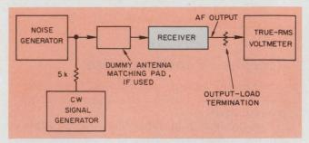
7. When only the audio output is accessible, this setup can measure receiver noise figure. The measurement is made on the linear portion of the quieting curve. Even an FM receiver has a small range of linear relation.
