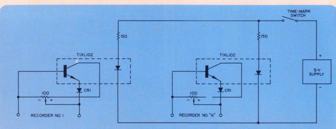
2. **Opto-isolators inject** the time-mark signals for N recorders. The potentiometer allows adjustment
