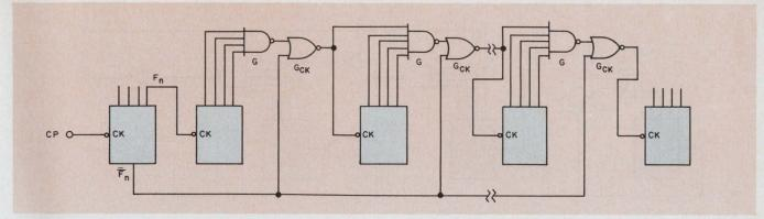
8. Synchronous sections can be used in a serial-enabled counter configuration (a). The first gate-inverter pairrequired for ripple sections-can be eliminated. The last stage makes a 1-to-0 transition as quickly as the first. If more sections are needed, then use synchronous sections in the circuit shown in Fig. 6.
