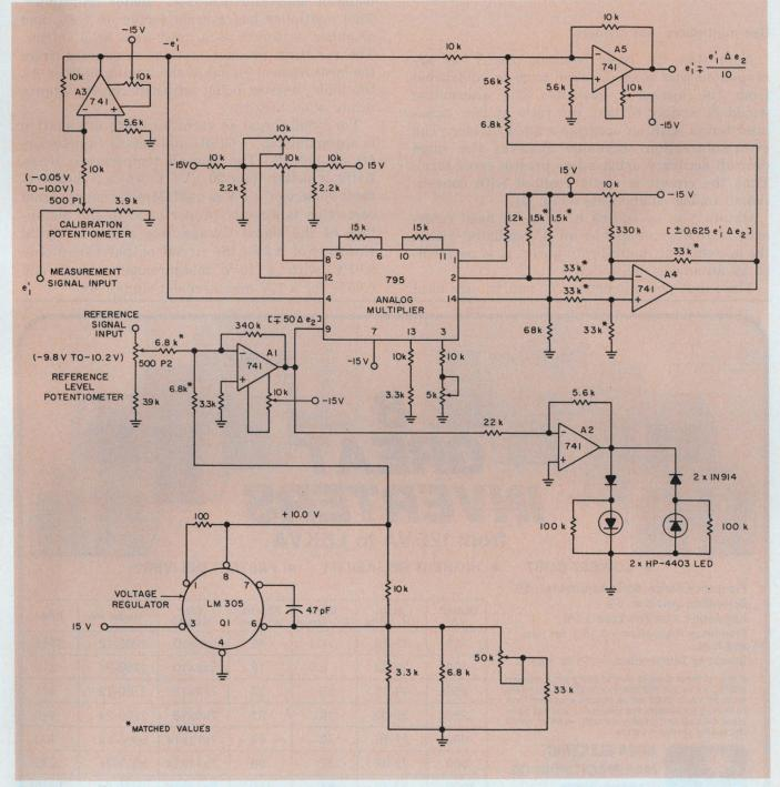
3. In the complete analog system that corrects the measured-signal level for variations in source intensity, voltage regulator  $Q_1$  acts as the reference voltage-source,
