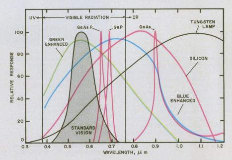
1. The spectral response of silicon has been modified by several manufacturers to improve shorter-wavelength sensitivity. One of Vactec's cells has the blue-enhanced curve while one of Sensor Technology's has the green.
