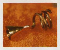
The flared input end of this channel multiplier, by Galileo Electrooptics, minimizes the device size.
