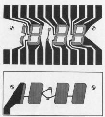
The comb-like structure in new fieldeffect liquid-crystal readouts from Ise Electronics more than doubles the viewing angle to 100° and eliminates the rainbow effect that's common in other liquid-crystal displays.
