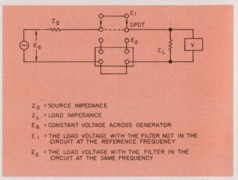
2. Accurate attenuation measurements below 1 MHz can be made using the method outlined in MIL-F-18327C.
