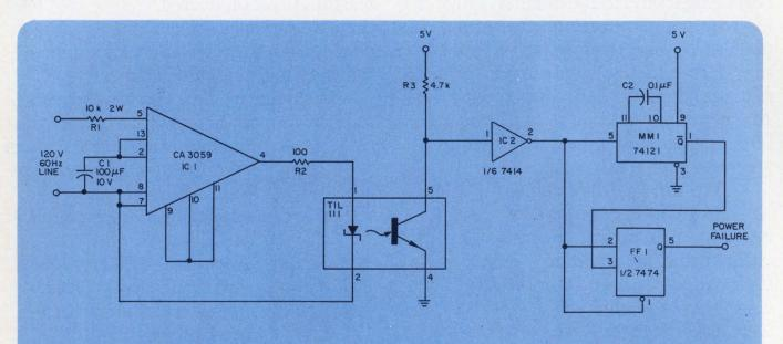
Zero-voltage switch minimizes reaction time of a power-failure detector.  $MM_1$  times out and sets  $FF_1$
