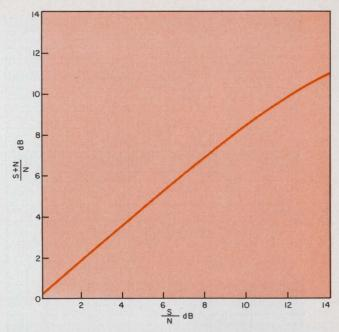
8. (S + N)/N to equivalent S/N ratio can be converted with this graph. Above about 10 dB, little error results if one is assumed equal to the other.
