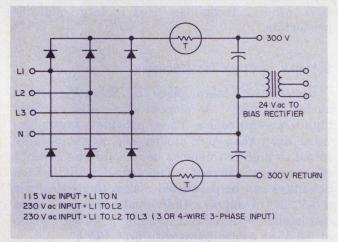
2. A three-phase bridge rectifies the input, which can be 115 or 230 V, single or three-phase. The thermistors limit line-inrush current.
