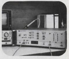
Pulse burst is generated upon receipt of trigger pulse. Length is determined by thumbwheel switches.
