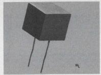
THE WL 451-T IS A HIGHLY LINEAR THERMISTOR. Using special semiconductor construction, the positive coefficient unit changes  $+4.93~\Omega/C^{\circ}$ . Special features include 1% tolerance, linearity  $\pm 1\%$  from -25 to  $+150^{\circ}$ C. Epoxy-cast in a .435" cube. \$9.50 (1-9) Western Laboratories 728 S. Marengo, Pasadena, CA 91106 213-793-0148 INFORMATION RETRIEVAL NUMBER 614
