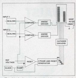
This block diagram for a dual linear bar graph shows you how simple the operation really is.
