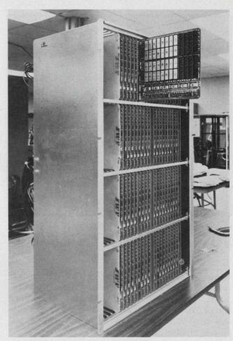
In addition to manufacturing chips, Advanced Memory Systems offers complete memory systems. The memory chips include 4-k dynamic RAMs and 1-k SOS arrays.
