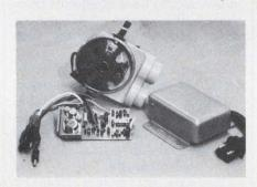
Electronic ignition hardware consists of distributor with trigger wheel, printed-circuit board with IC, sensor coil (mounted on distributor housing) and enclosure.
