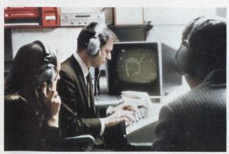
Synthetic speech is being produced with 1/50th the previously required digital information. The digital coding scheme developed at Bell Laboratories is ideal for transmission over a fiber-optic link. The screen shows a graphic representation of synthetic speech.
