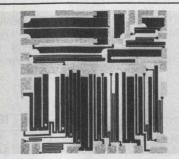
Complete Functions Offered on a Chip. High density monolithic thin film processing offers exceptional resistive performance for hybrid asresistive performance for hybrid assembly. 250 standard variations available to .01% accuracy, tracking to 0.5ppm/°C. Analog Devices, Inc., Route 1 Industrial Park, P.O. Box 280, Norwood, Massachusetts 02062. Telephone: 617/329-4700.
