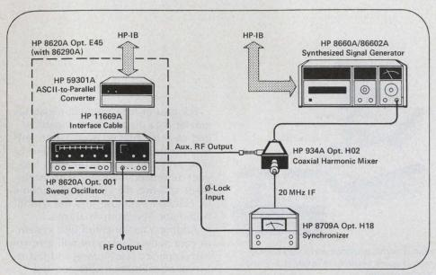
Synthesizer accuracy to 18 GHz is easily obtained via the HP-IB.
