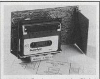
MEMODYNE Incremental Digital Cassette recorders read, write, store alpha-numeric data at 50 cps in ASCII or 8-bit parallel. 72,000 character capacity. Low power (CMOS) for data logging, off-line terminals, microprocessors. Interfaces w/wide variety. Lit. avail. Memodyne Corporation, 369 Elliot St. Newton, Mass. 02164 617/527-6600 telex 922537
