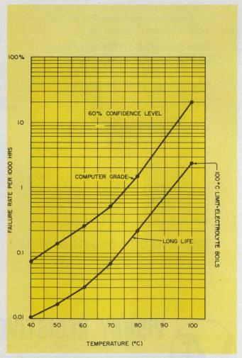
1. An electrolytic capacitor's core temperature strongly affects its failure rate. Core temperature can be much higher than ambient, when ripple current flows.
