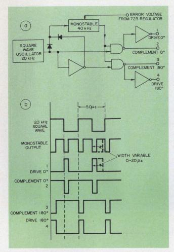
7. To derive the four signals to drive the Darlington bridge, the one-shot output is "mixed" with the 20-kHz clock in two NAND gates (a). The resulting waveforms consist of two out-of-phase signals and their complements (b).
