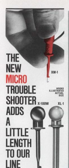
(1.75" - 4.45 cm) long and VERY little weight (less than 1 gram). Ideal for difficult IC testing. Connect DIRECT to IC...Reduce resistance build-up. Same high quality construction as our models X-100W, (2.25" - 5.7 cm) and XL-1, (5"-12.7 cm): Durable heat and chemical resistant nylon body, Gold-plated Beryllium copper contact, Stainless steel spring. Single contact point makes fast, safe, short-free connections... assures accurate readings.
