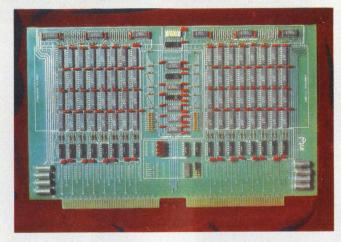
16-k bit CCD memory chips—Intel's 2416—are the main element of a 1-Mbit prototype board. Of all the packages, 30% provide support circuits.
