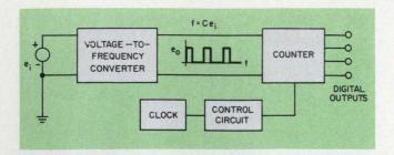
1. The output of a v/f converter can be encoded by a digital counter to simulate an a/d converter.
