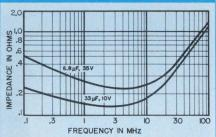
Dual in-line plastic package for mechanical protection and increased reliability. Preferred ratings are 6.8  $\mu$ F @ 35 V, 15  $\mu$ F @ 20 V, 22  $\mu$ F @ 15 V, and 33 μF @ 10 V. Operating temperature range, -55 C to +85 C.
