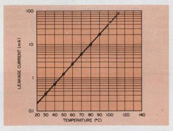
3. Leakage current doubles every time the core temperature rises about 10 C.
