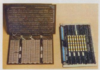
Memory boards employ 512-bit CMOS static RAMs— American Microsystems' S2222. The boards are used in Rolm's Rugged Nova system.
