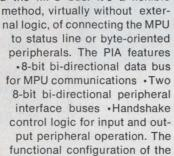
PIA may be changed by the MPU during system operation.
