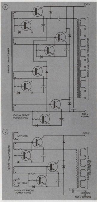
12. Power stage for a 1000-W output (a). Commutating diodes and other circuitry shunt the output-transformer inductive currents to ensure proper turn-off. If only 500 W are needed, a half-bridge connection can be used (b).
