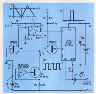
If clocked control of the discharge time is used, accuracies to within 0.01% are obtainable.
