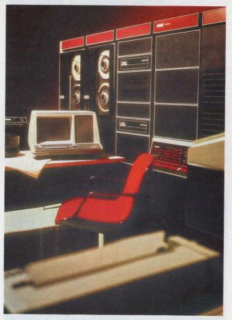
Digital Equipment Corporation's new midicomputer, the PDP 11/70, employs a special memory architecture in which a 2 k byte bipolar cache memory acts as a buffer between main memory and the unit's general purpose registers. 32-bit internal data paths carry data to and from the cache memory, permitting data transfers between memory and registers to approach the 300-ns execution time of the central processor.
