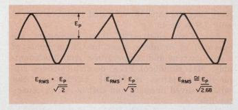
2. The approximate rms value of ripple current can be calculated from the current's peak value and a constant determined from the waveshape.
