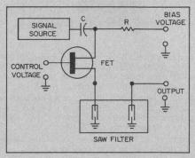
achieved by use of a system made up of several transducers, each of which receives the input signal via a separate FET. The frequency response is shaped by adjustment of the phase relationships of control voltages applied to the transistor gates. A single wideband transducer receives the acoustic wave for output.
