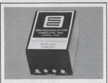
The ''75WS15T'' provides  $\pm 15$ Vdc @ 150mA and an isolated 15Vdc @ 200mA with rem. sense. Sense current 200  $\mu$ A; Tempco 0.002%/°C; 1500V isolation; current foldback on all outputs, 0.V.P. on X-Ducer supply; Price \$196.00; Del 2 wks. Other models avail—contact Semiconductor Circuits, Inc., 306 River Street, Haverhill, MA 01830, (617) 373-9104 INFORMATION RETRIEVAL NUMBER 611
