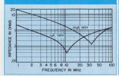
Proven multi-layer construction. C0G(NP0) and X7R temperature characteristics. Preferred ratings are .01, .047, and .1 μF @ 100 WVDC. Operating temperature range, -55 C to +85 C.
