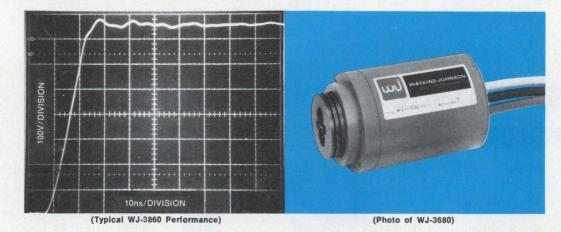
Now available from Watkins-Johnson, this Electron Bombarded Semiconductor (EBS) has been designed for high-speed, short-delay, fast-rise-time switching and modulation applications.
