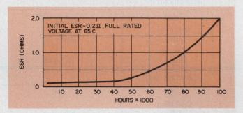
4. A capacitor's ESR increases with the unit's age, mostly because of loss of electrolyte.
