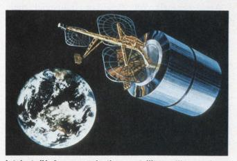
Intelsat IV A communications satellites will use timedivision multiplexing for maximum channel capacity. TDMA also makes the satellite an efficient data-communications vehicle. Shown here is the current generation of satellites built by Hughes Aircraft.
