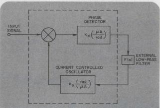
1. PLL circuit's performance can be improved by use of an active external low-pass filter that provides gain in addition to filtering.
