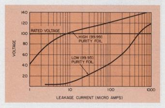
5. Leakage current is strongly affected by the purity of the aluminum foil used in manufacture.
