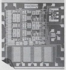
CMOS silicon-on-sapphire circuits, such as this 4008-type 4-bit adder from Rockwell International, are undergoing tests to develop radiation-hardened MOS/LSI circuits. This chip has 170-transistor complexity and a chromium-doped gate oxide.
