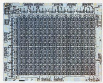
A 1024-bit CMOS static RAM, Intersil's IM6508, offers 250-ns access time over the full temperature range with a 5-V supply. Access drops to 100 ns at 10 V.
