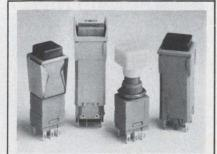
S190/S410 Switchlights. Low cost 2 Form C Mom. & Alt. action; Dual wiping contacts. Rating 100,000 cycles @ 2 amp res., 0.5 amp ind., 30 VDC & 125 VAC. Quick connect & solder terminals. Snap-in & rear panel mount. 10-amp power switch UL listed. Varied lens shapes. Clare-Pendar Co., Box 785, Post Falls, ID (208) 773-4541
