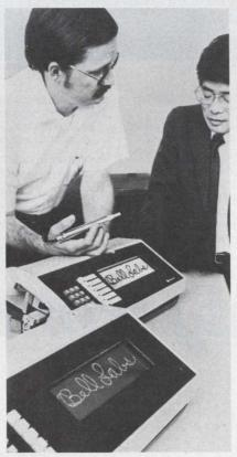
Flat-screen plasma panel transmits photographs, drawings and writing to remote panel by telephone wire.
