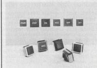
Touch Activators for solid-state switch circuits eliminate pushing, pulling, or flipping of switches. No moving parts; high reliability. A mere touch of finger activates switch circuit. Interface with CMOS, TTL, DTL, and HTL. Snap-in panel mounting. Lighted or unlighted. Master Specialties, 1640 Monrovia, Costa Mesa, Calif. 92627.
