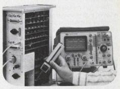
With dual-delayed sweep, two markers select time period to be measured and a proportional voltage output is provided for DVM readout.
