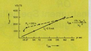
Output voltage of a regulated high-voltage power supply is controlled by variable-resistor R<sub>1</sub>.
