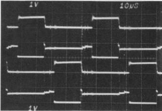
Signal and phase relationships (top to bottom): DM8601, MC4024 and DM 8090 outputs at full load, nominal line.
