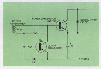
9. Turn-off current,  $I_{\rm B2},$  is provided by a transistor clamp arrangement at the base of the Darlington.
