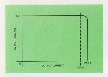
5. Regulation provides a constant-voltage output up to the overload point (250 A) and then goes into a constant-current mode to 0  $V_{\bullet}$
