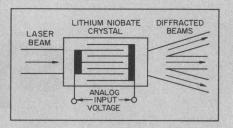
tion of voltage to the electrode system terminals produces spatially periodic variations in the refractive index of the crystal. As a result, a laser beam passing through the crystal is modulated in intensity, as different orders of power are diffracted in controlled directions.
