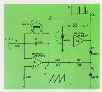
3. Higher precision (0.1%) v/f converters use a comparator-controlled reset circuit.
