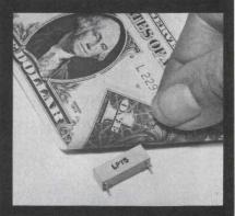
High contact resistances, changing resistances and excessive contact bounce are usually traceable to the high molding pressures and temperatures used in making DIP reed relays. High unit costs and long delivery times are inherent in the DIP reed relay molding processing itself.
