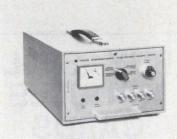
Atomic Frequency Standard Model FRT for Lab/Field. Output  $10\text{-}5\text{-}1\ 0.1$  MHz, Short Term Stability  $<1\text{x}10^{-11}$   $\tau=1\text{s},<1\text{x}10^{-12}$   $\tau=100\text{s}.$  Drift typ  $1\text{x}10^{-11}/\text{M}.$  Coupled with Receiver-Controller EFR. Sync to Standard Freq absolute freq parts in  $10^{12}$ . Efratom Calif., Inc., 3303 Harbor Blvd., E1, Costa Mesa, Ca. 92626 (714-556-1620)
