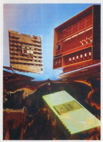
The first 16-bit microprocessor on a single chip is the Pace from National Semiconductor. It has a 45-instruction set that cannot be modified. Instruction cycle time is typically 10  $\mu$ s. Shown also is the Pace microcomputer card prototyping systems.
