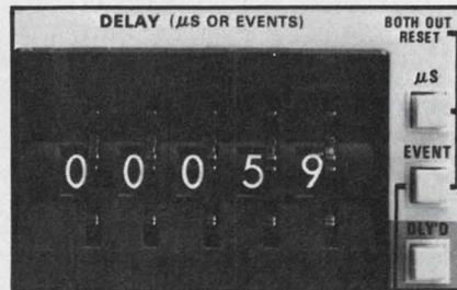
Then you can study any portion of the waveform in detail by adjusting the thumbwheels and increasing the sweep speed.
