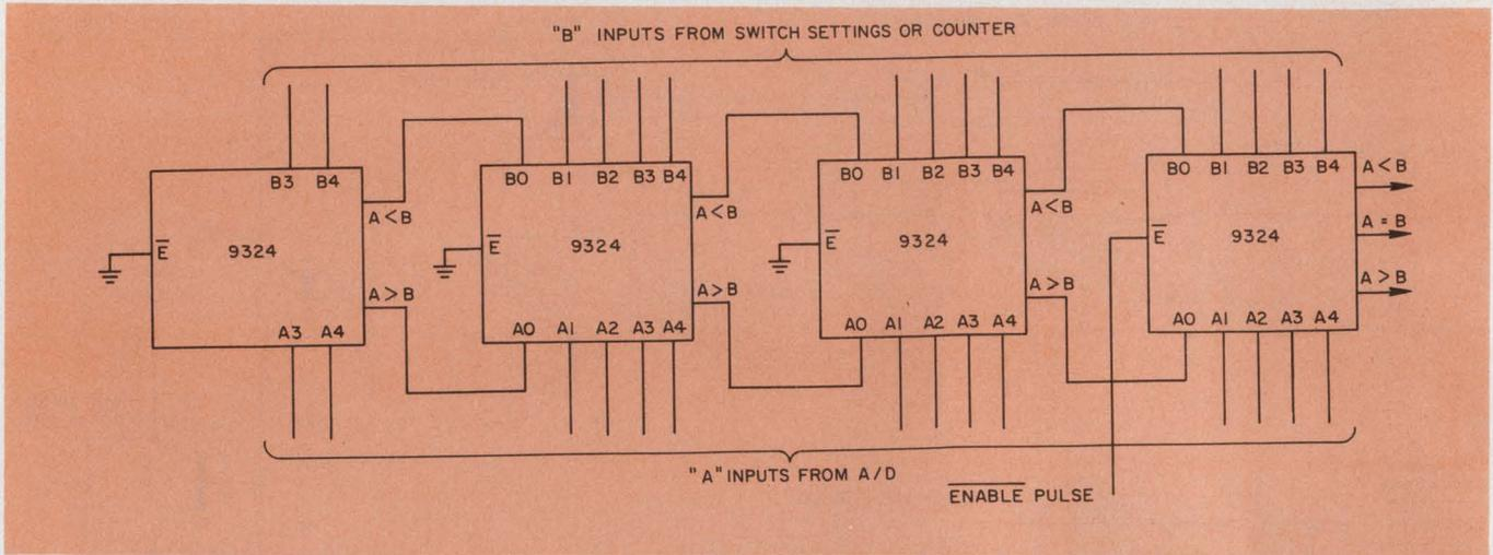
10. Four 5-bit comparators are connected to form the 14-bit digital circuit that compares the converter's out-
