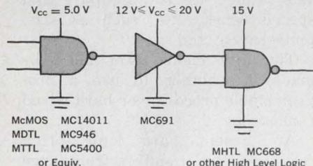
The MC696 Dual Interface Unit, Line Driver/Receiver offers flexible hysteresis capability for design variety. And has low output impedance of  $\approx 20$  ohms in LOW state.
