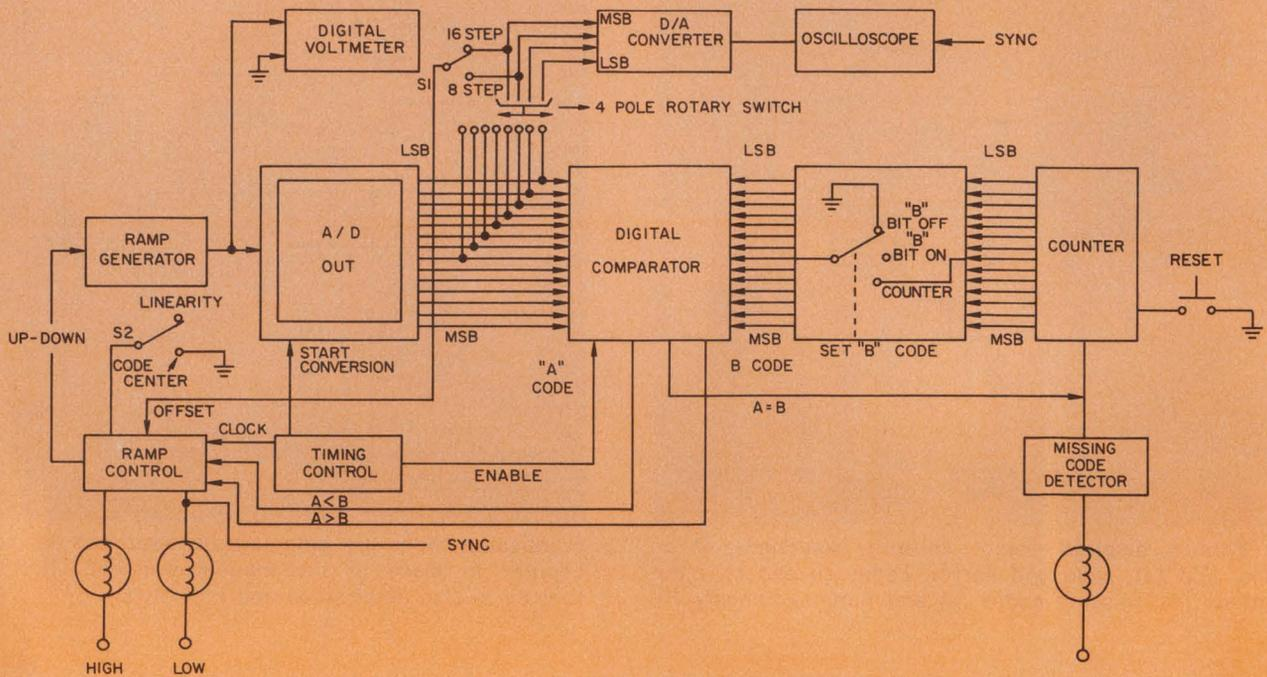
7. The complete a/d converter tester, with all additions and modifications, can determine converter errors in several ways. Code centers are measured with the digital
