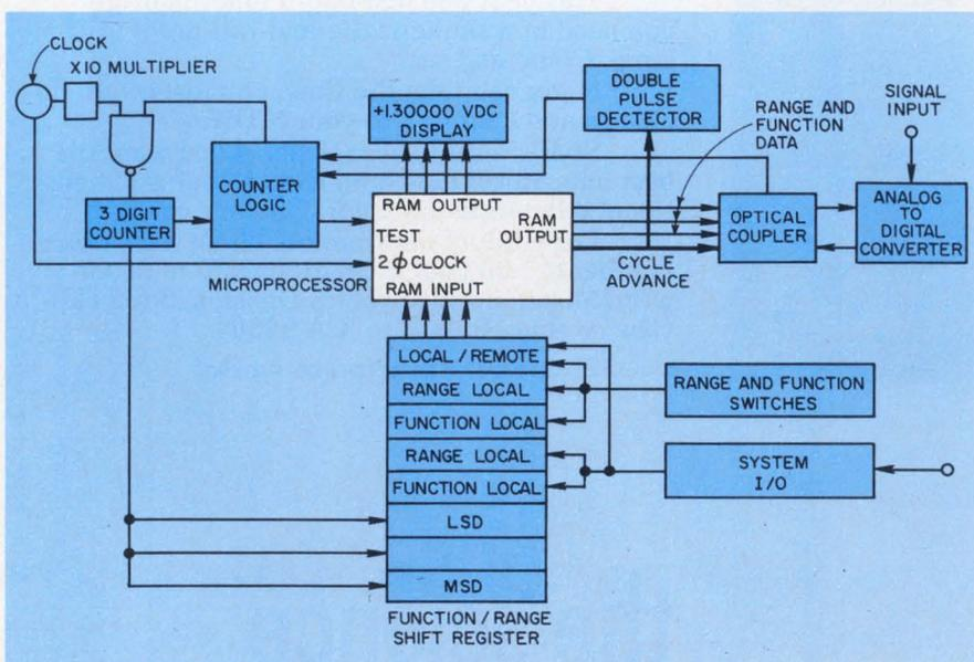
In the first LSI microprocessor-based digital voltmeter, from Systron Donner, the computer-on-a-chip, plus memory ICs, replace all the digital logic ordinarily used in such an instrument. Benefits include self-calibration.
