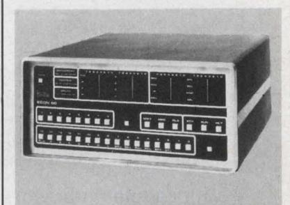
**ELCON 80 DEVELOPMENT SYSTEM** Emulation of 8080 expands design aids to simultaneous 8080 register display • Operation from dc to 2Mhz • Utilities in microcode • Breakpoint and I-C-E capability • TTY interface • High density Prototype boards and power supplies options • 15-30 day. SANTEK SYSTEMS, 6645 Convoct Ct., San Diego, Ca. 92111 (714) 560-1101
