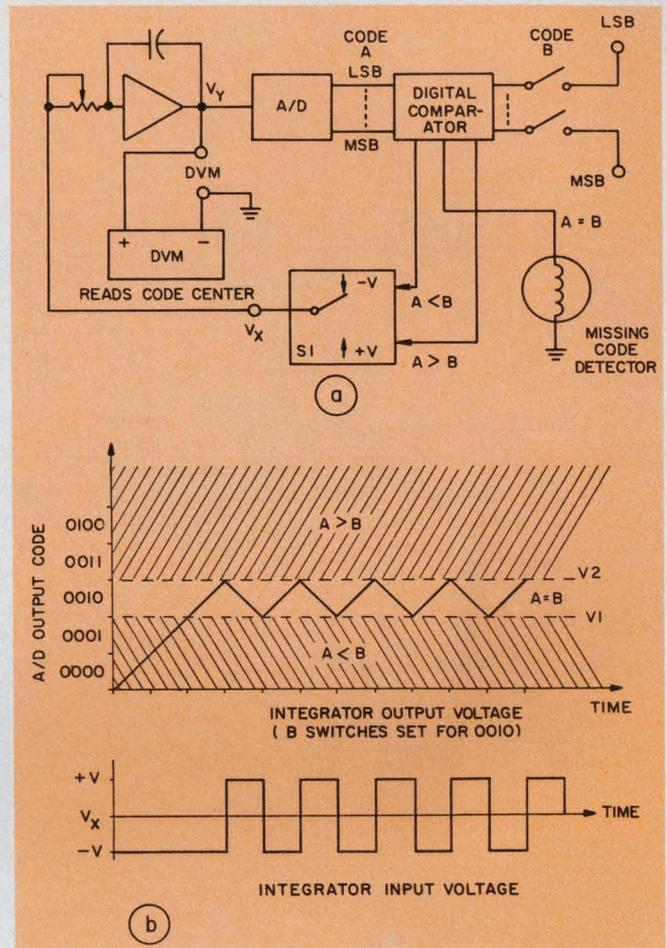
2. Code centers can be determined by use of a digital comparator and feedback to an integrator (a). The integrator's output ramps up or down, depending on where the comparator sets the solid-state switch (b). The manual switch is set by the user to an arbitrary code.
