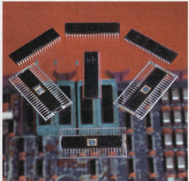
Western Digital produces a chip set that is used by Digital Equipment Corp. as the heart of the board-level microcomputer, the LSI/11. These chips allow Digital Equipment to market a 16-bit PDP-11 minicomputer on a board.
