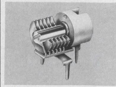
**High performance Type "T" sub-miniature machined-plate capacitors.** Rotors and stators machined from solid brass extrusions provide excellent stability and uniformity. High Q, low temp. coefficient (plus 30 ± ppm/°C). Available in horizontal and vertical tuning for PC and stripline mounts. E. F. Johnson Co., Waseca, MN., (507) 835-5222.
