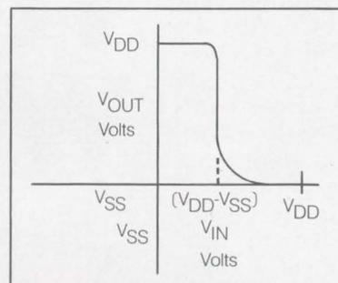
This CMOS transfer characteristic for single level gate functions is for all CMOS logic families. It is the commonality of this characteristic which is the basis of CMOS inter-family compatibility.
