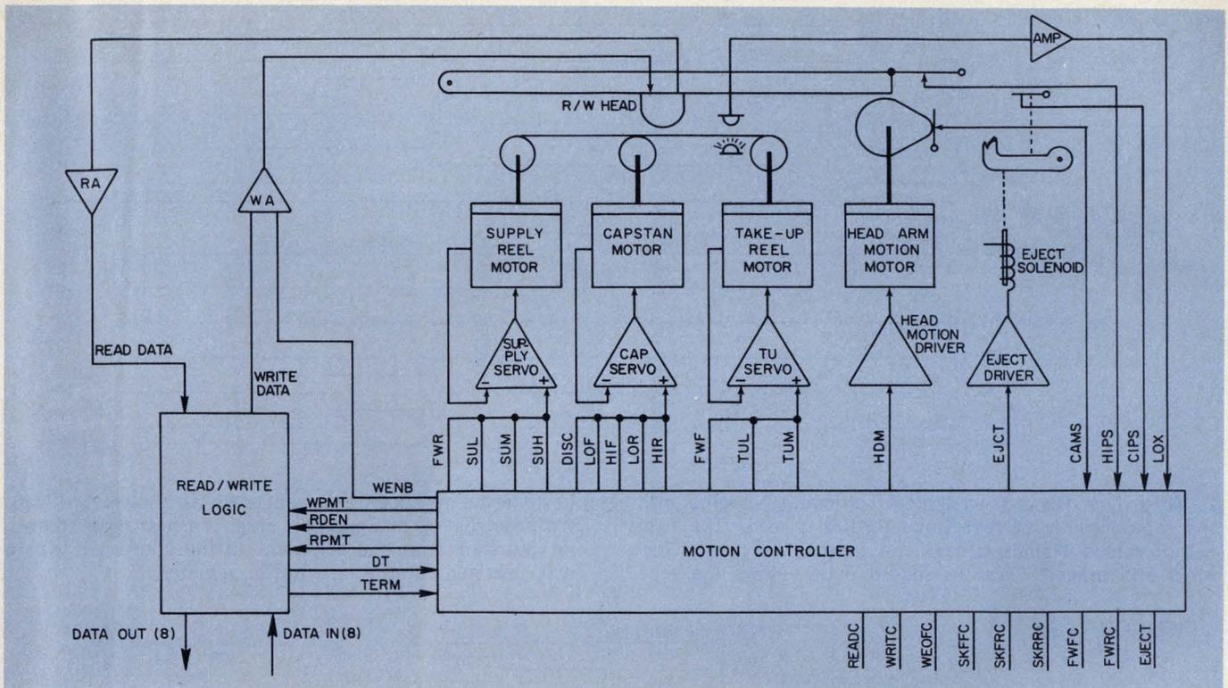
1. A cassette-tape drive system uses a programmable controller consisting of read-only memory and an MSI-
