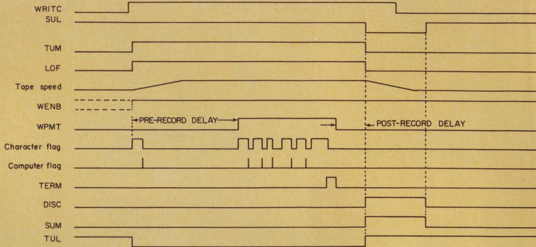
2. **Write One Record**—a typical command—begins with the tape initially at rest (tape torque is low). The first set of raised signals causes the tape to be moved forward and erased. This pre-record delay allows the tape
