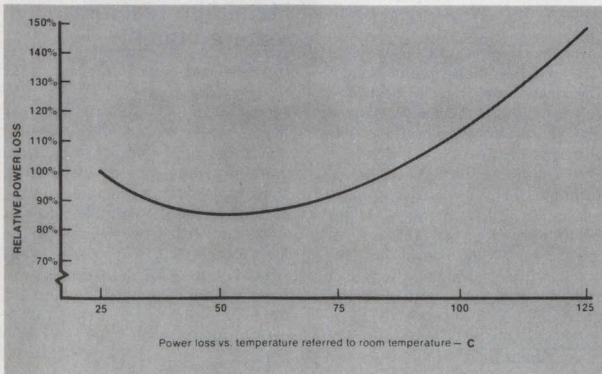
Power loss vs. temperature referred to room temperature — C
