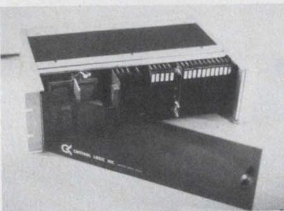
A modular microcomputer development system is available from Control Logic. The microcomputer chips and various I/O, memory and other support chips are each packaged on small PC boards. The boards can be housed in the Control Logic chassis and used together to form a microcomputer system.
