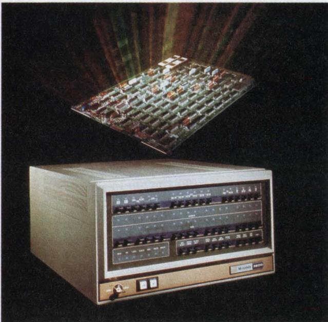
Both **board-level microcomputers** and **full scale minicomputers** are produced by a few companies. Microdata shows the full-scale 3200 and the board-level Micro-One. The microprogrammable Micro-One can emulate any other microcomputer on the market.
