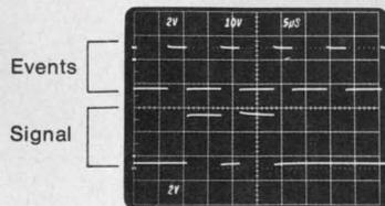
The 5B31 has a digital delay system—a crystal-controlled clock, a digital counter, and a circuit that eliminates 1-count ambiguity—that introduces no more than 20 ns of jitter at any sweep speed. So the 5B31 will have little effect on the stability of your display, even at very high sweep speeds.
