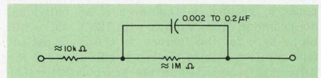
6. **An equivalent circuit** of the skin's contact impedance accounts for tissue and fluid resistance and capacitance.
