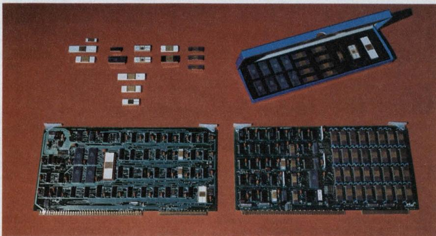
Intel's popular 8080, 8-bit n-channel MOS microprocessor can also be bought at many levels of integration. The chips are available to designers who choose to assemble their own boards. Or a small prototyping kit can be purchased. In addition larger boards are sold, with all the associated circuitry to make a complete CPU or add-on memory boards.
