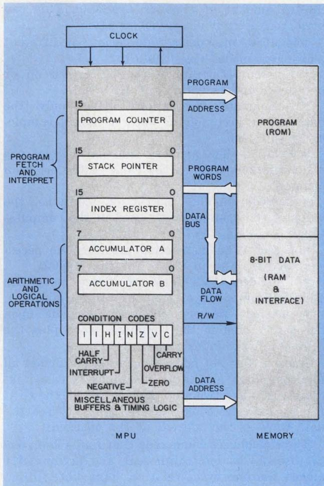
2. Inside the MPU are the different counters and registers that let you separately keep track of both the program and data. And, correspondingly, the programmer treats memory as if it were composed of two parts—a data or variable section and a command or instruction section. Also included are the logic circuits and control gates needed to do all the arithmetic operations.
