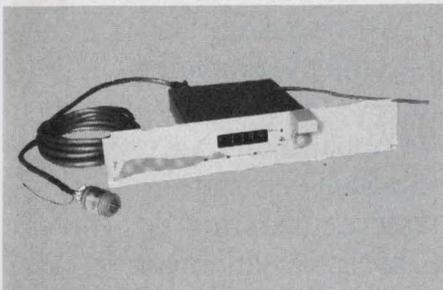
**ABSOLUTE ENCODER**— $\pm 1$  Part in 3600 System Accuracy, Electro-Magnetic Transducer + LED Display + BCD, Binary, and DC Output—Infinitely Adjustable Scale Factor (0 to 9999)—Hi Noise Immunity—Zero Offset—Single and Multi-Channel Units From \$375/Axis (1 pc.) Computer Conversion Corporation, East Northport, NY 11731 516-261-3300
