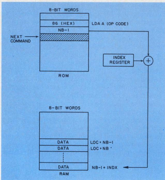
3. When the op code LDA A is given, the byte of binary data following the instruction is added to the index register information to supply the address of the data needed by the op-code instruction.
