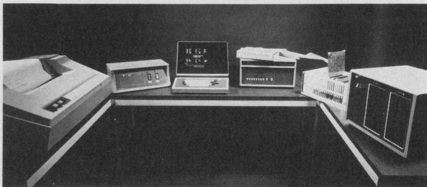
**A complete microcomputer software-hardware development package** is contained in Intel's MDS system. Its multiprocessor configuration permits design, development and debugging of systems based on the Intel 8080.
