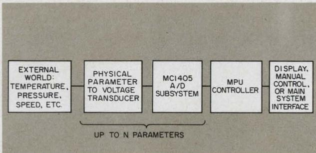
5. In a typical application, the  $\mu\text{P}$  controlled system monitors physical parameters, such as pressure, and provides a digital readout of a desired value.
