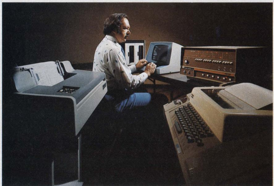
**Microprocessor software programs can cost orders of magnitude more than the hardware.** Programs can be generated using only a teletypewriter and a time-sharing service (top). But the slow speed of this system limits the lines of instruction code produced per hour. Fast, cost-effective software generation requires an investment like that of the National Development System (bottom) that incorporates an IMP-16P, an interactive CRT, a high-speed printer, a floppy-disc system and a teletypewriter.
