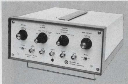
**Model A-101 Ultrasonic Pulser/Receiver** drives piezoelectric transducers. High energy negative spike output variable from -50 to -350 volts into 50 ohms. Pulse repetition rate adjustable from 100 Hz to over 10 kHz. Pulse risetime better than 15 nsec., output pulse monitor, adjustable damping. TTL-compatible external trigger, sync. Low noise receiver amplifier has selectable gain, 15 MHz bandwidth, switchable high-pass filter. MetroTek, Inc., P. O. Box 101, Richland, WA 99352, (509) 946-4778.
