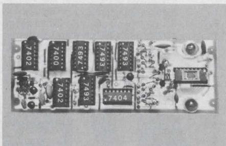
**Low Cost Image Sensing Module** contains a 1024 element (32-by-32) image sensor and all support circuitry on a single pc board. Digital video output may be displayed directly on an oscilloscope. Complete module (SE1024W) is \$150. Kit (SE1024K) is \$90. Cromemco, 26655 Laurel, Los Altos, CA 94022.
