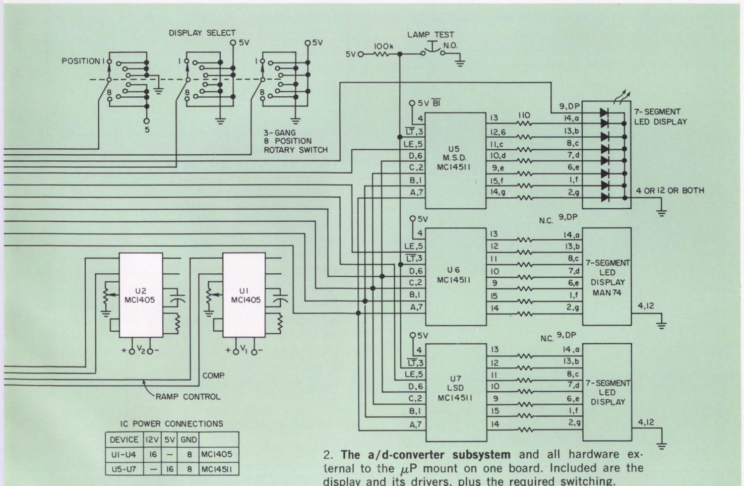
2. The a/d-converter subsystem and all hardware external to the  $\mu$ P mount on one board. Included are the display and its drivers, plus the required switching.
