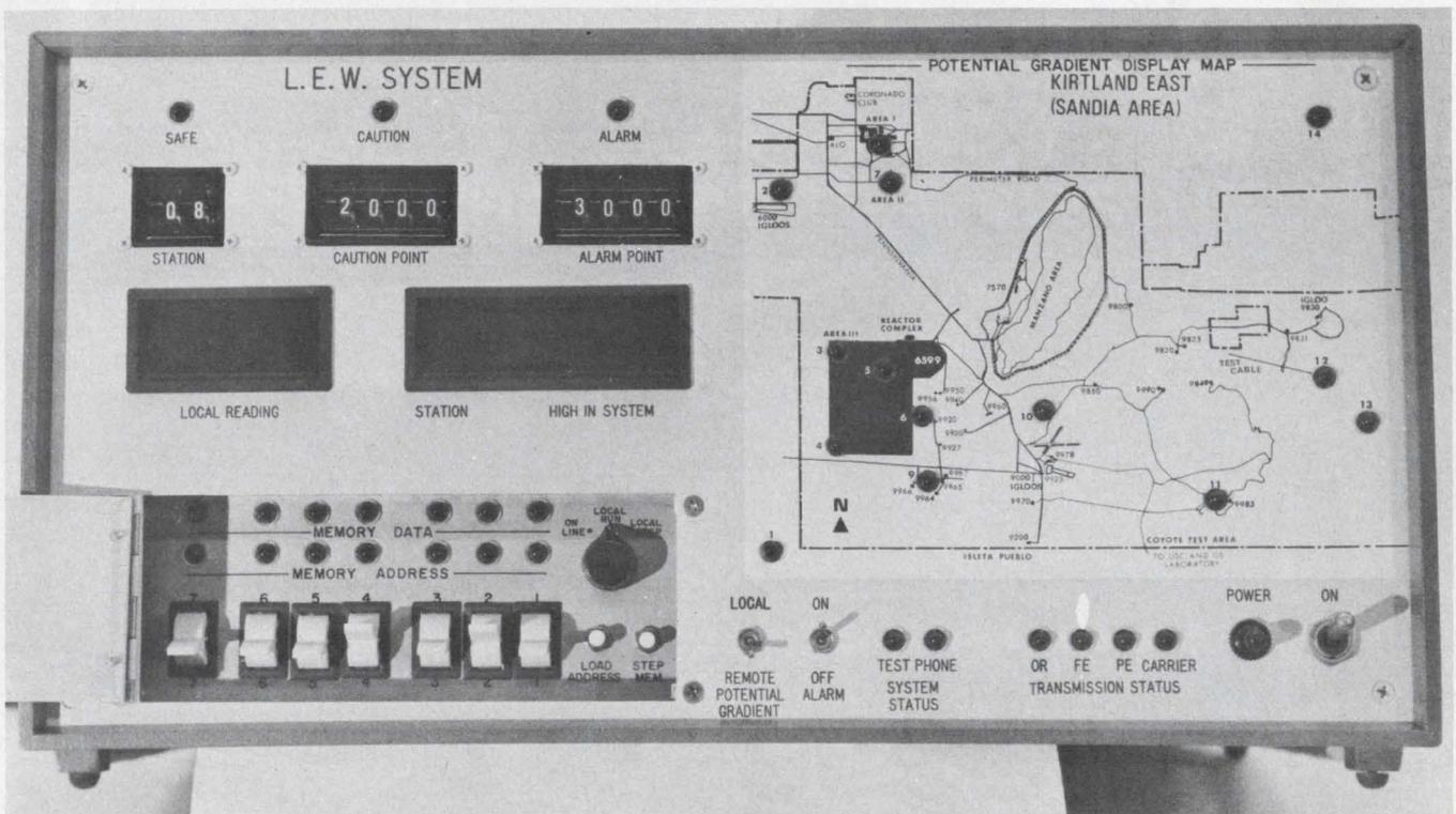
Display panel of on-site early-warning system equipment has a map with sensors pinpointed by warning lights.
