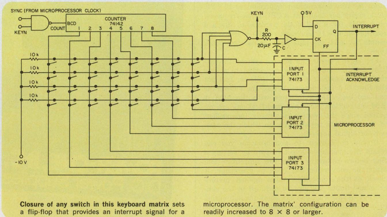
Closure of any switch in this keyboard matrix sets a flip-flop that provides an interrupt signal for a
