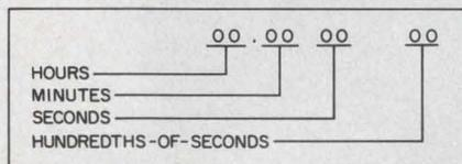
To start the clock function, press the CHS key. Pressing the CHS key again will stop the clock without resetting the display to zero. (To reset the display to zero, press the CLx key.)
