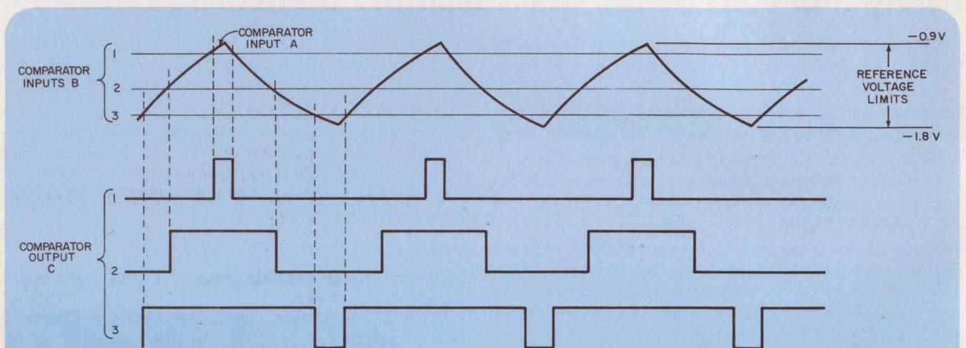
2. The duty cycle is controlled by comparator input B from the reference-voltage source.
