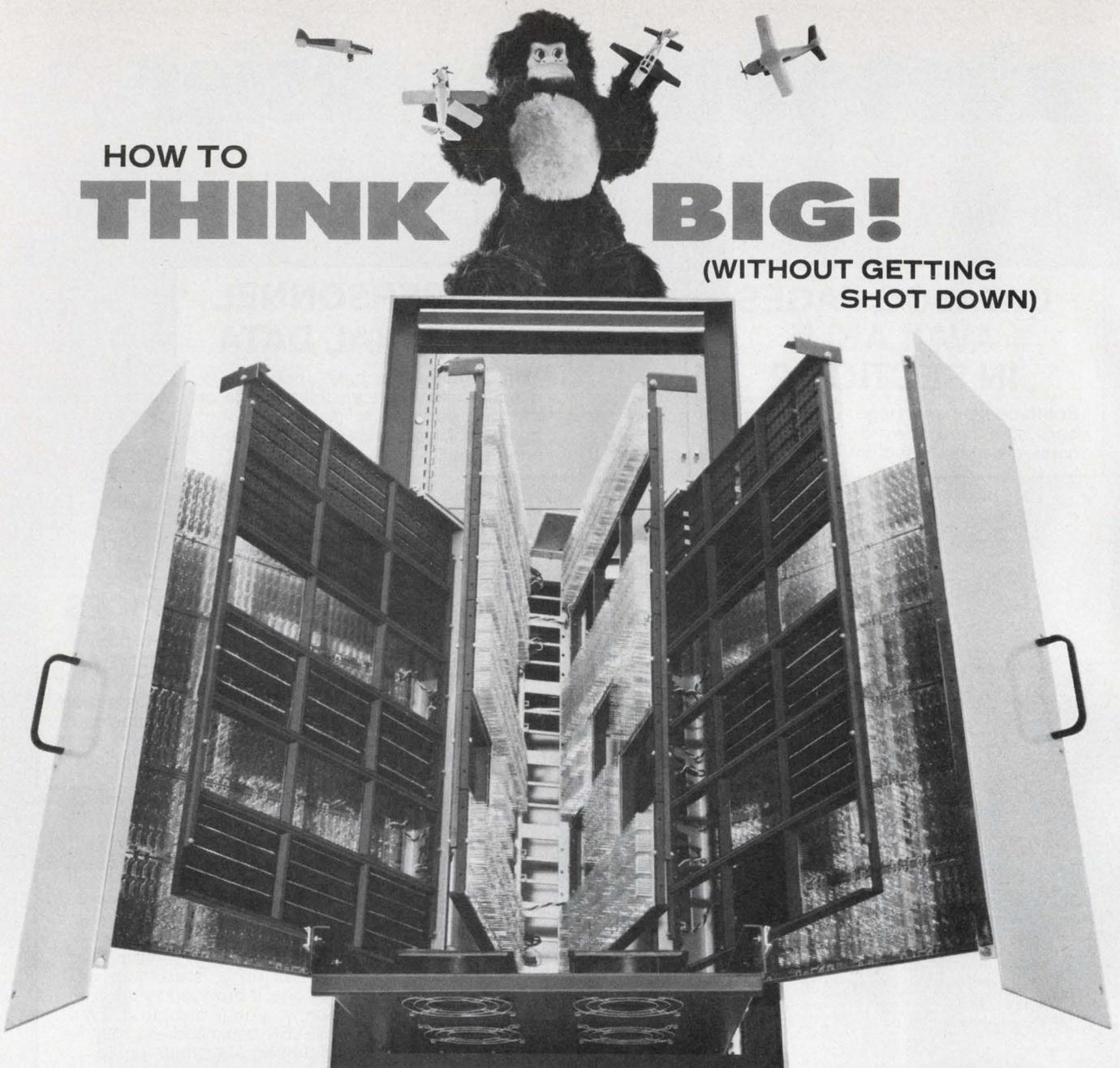
**XLP 6x6**—our largest standard system packaging assembly—can hold over 5100 ICs. You can select from 98 standard modular wire wrap boards to include microprocessor sections, low noise sections, economy boards, ECL, memories, whatever you need.
