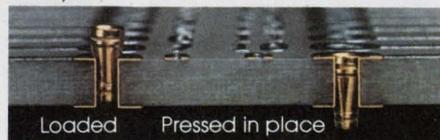
tacts an hour, which includes pressing them into place using a standard hydraulic press.
