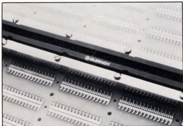
5. Burndy's 300-contact Ziflex connector combines surface-mounting technology at the connector-backplane interface with ZIF technology at the interface of the card edge and its connector.
