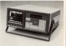
channels at 200 MHz, both synchronously and asynchronously. This mode includes eight clock inputs with full Boolean, master-slave, or double-edge clocking. In the split mode Paladin offers 80 channels of 100-MHz synchronous data collection along with 20 asynchronous channels. In the high-speed mode the system supplies 10 asynchronous channels at 1 GHz and 20 asynchronous channels at 500 MHz. Multiple modules can be connected together.
