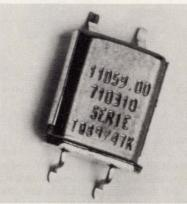
lator circuit with an internal AT-cut crystal. The unit operates from 625 kHz to 24 MHz and is mounted in a 28-pin PLCC. It delivers a square-wave output with TTL fanout of 10, or 50 pF of high-speed CMOS loading.
