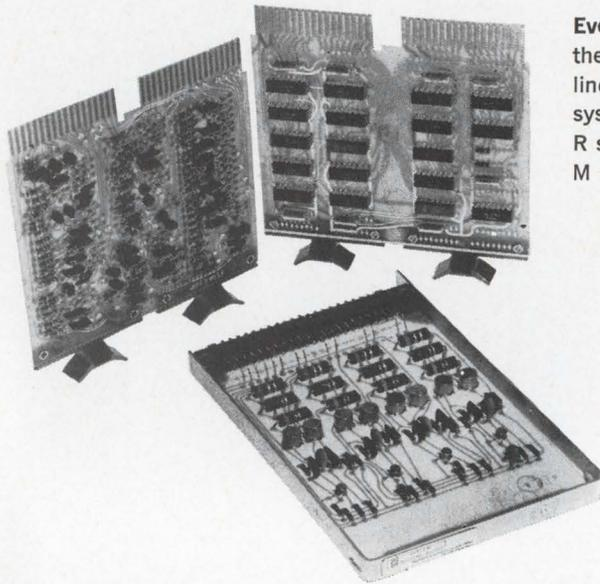
**Evolution.** Three stages in the development of DEC's line of circuit modules; the system modules at bottom, R series at left, and new M series at right.
