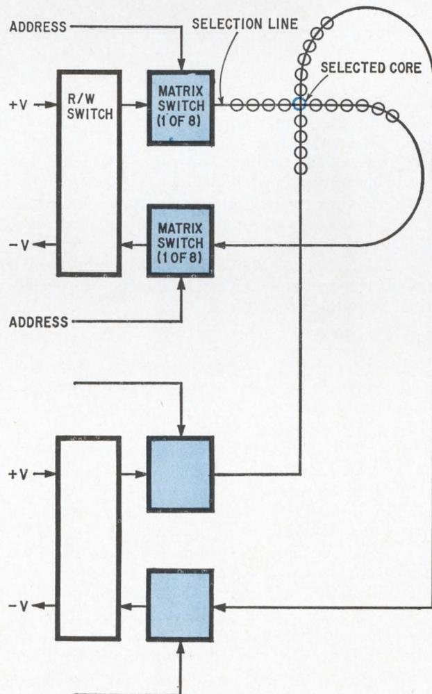
**Matrix switch.** Four diodes and a transistor replace a pulse transformer, helping to reduce the size of the PDP-8/I memory.
