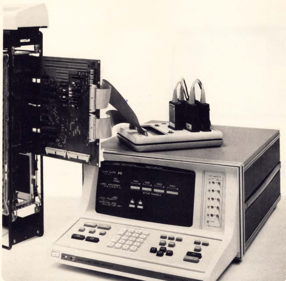
Shown here is an HP 1027A PDP-II UNIBUS Interface on an extender board plugged into a minicomputer for tests with a logic analyzer. Also shown is a 10277A (on the 1610A logic analyzer) general purpose interface which interconnects through probe pod "buckets" and two 40-pin ribbon connectors.
