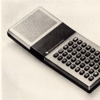
Fluent. Talking language translator, shown here in prototype without display, is calculator-sized and powered by four AA batteries.
