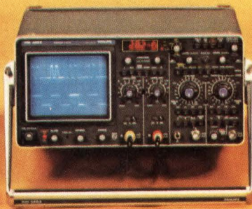
PM3263 100MHz Microprocessor-Equipped Scope with Digital Delay
