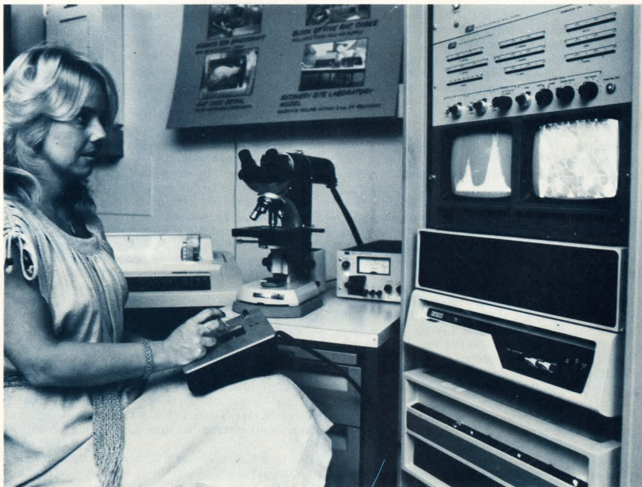
Making a muscle. To be described in a medical session at Wescon is this system from Caltech's Jet Propulsion Laboratory. With its assistance, an operator can locate and measure muscle fibers under the microscope.
