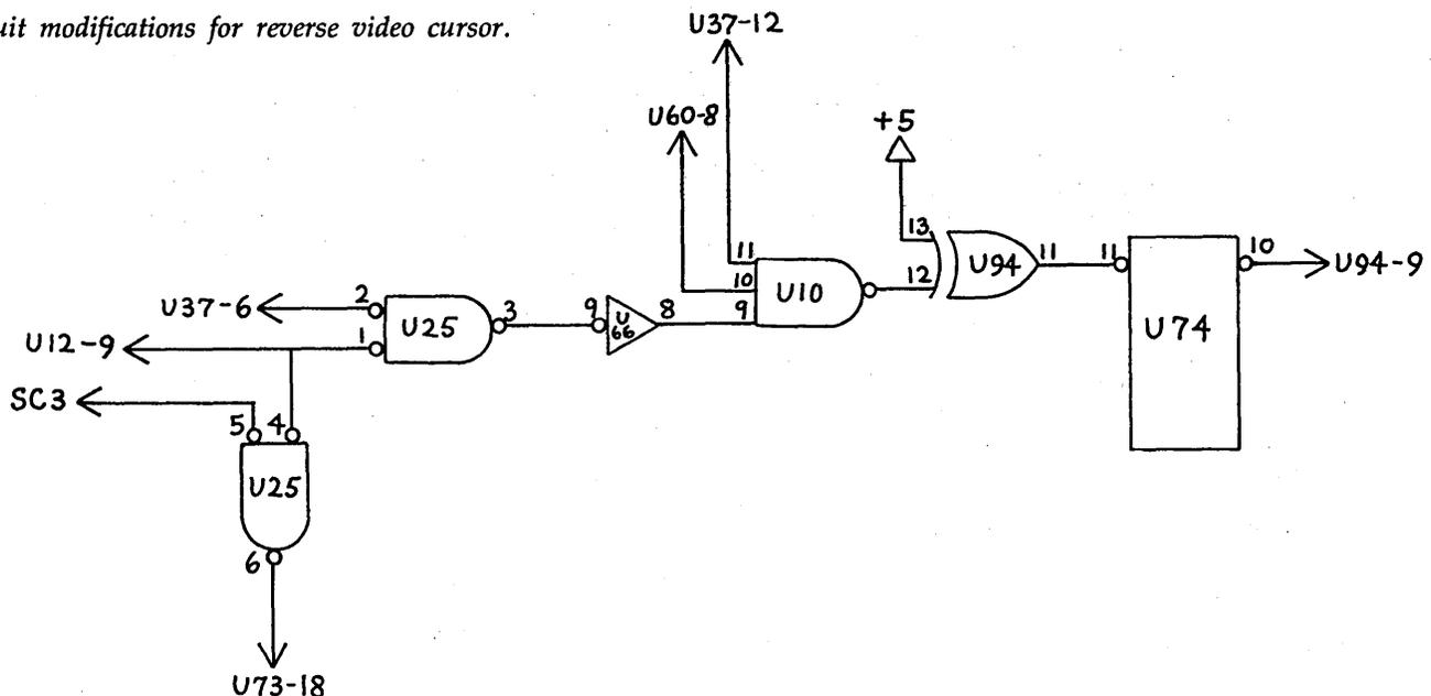
the video signal fed to your monitor. By connecting pin 10 of U74 to pin 9 of U94 we will produce an inverted character whenever bit 7 is set.
